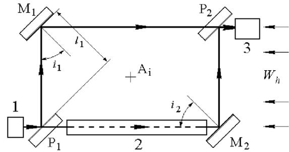
Figure 3: The schema of an optical interferometer
