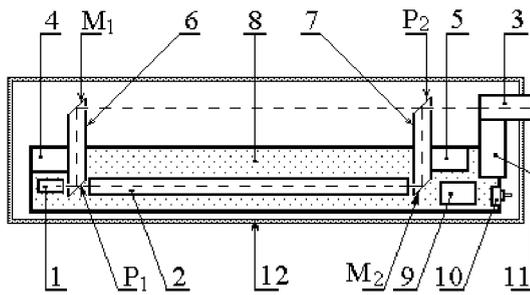
Figure 5: The interferometer structure
