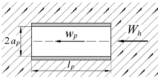
Figure 1: A tube in a gas stream
