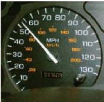
**FIGURE 2-8** Car speedometer showing mi/h in white, and km/h in orange.
