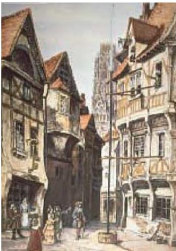
**FIGURE 13–12** A water barometer: a full tube of water is inserted into a tub of water, keeping the tube's spigot at the top closed. When the bottom end of the tube is unplugged, some water flows out of the tube into the tub, leaving a vacuum between the water's upper surface and the spigot. Why? Because air pressure can not support a column of water more than 10 m high.
