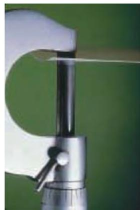
**FIGURE 1-8** Example 1-6. Micrometer used for measuring small thicknesses.
