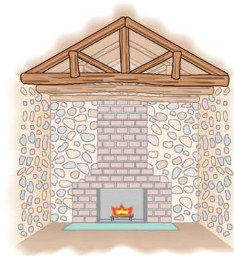
FIGURE 12-26 A roof truss.
