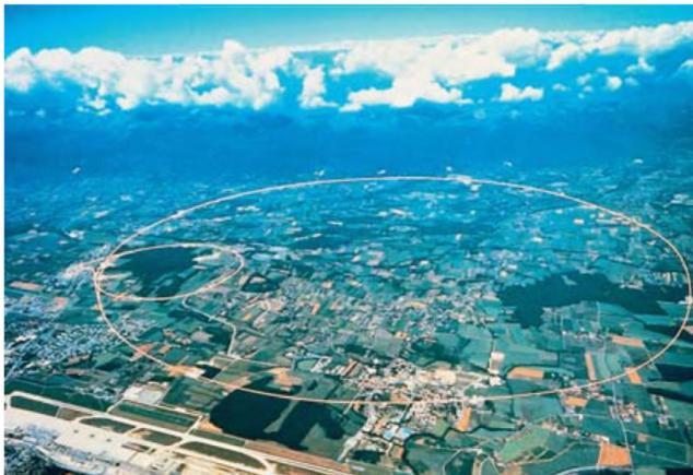
**FIGURE 43–5** The large circle represents the position of the tunnel, about 100 m below the ground at CERN (near Geneva) on the French-Swiss border, which houses the LHC. The smaller circle shows the position of the Super Proton Synchrotron that will be used for accelerating protons prior to injection into the LHC.
