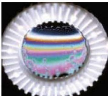
Farther down, with increasing thickness  $t$ , a path length  $2t = 510 \text{ nm}$  corresponds nicely to  $\frac{3}{2}\lambda$  for blue, but not for other colors, so we see blue ( $\frac{3}{2}\lambda$  path difference plus  $\frac{1}{2}\lambda$  phase change = constructive interference). Other colors experience constructive interference (at  $\frac{3}{2}\lambda$  and then at  $\frac{5}{2}\lambda$ ) at still greater thicknesses, so we see a series of separated colors something like a rainbow.
