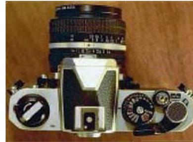
**FIGURE 33–21** On this camera, the  $f$ -stops and the focusing ring are on the camera lens. Shutter speeds are selected on the small wheel on top of the camera body.
