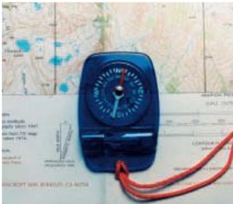
**FIGURE 27-6** Using a map and compass in the wilderness. First you align the compass case so the needle points away from true north (N) exactly the number of degrees of declination as stated on the map (15° for the place shown on this topographic map of a part of California). Then align the map with true north, as shown, *not* with the compass needle.
