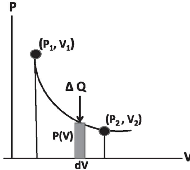
Figure 22.4 During an infinitesimal change by  $dV$ , the work done by the gas is the shaded area  $dW = PdV$ . If this were an isothermal process, some heat  $\Delta Q$  would flow in from the reservoir to keep  $T$  and  $U$  constant. For a finite process the work done is the area between the  $V$  axis, the graph  $P(V)$ , and the vertical lines at  $V = V_1$  and  $V = V_2$ .
