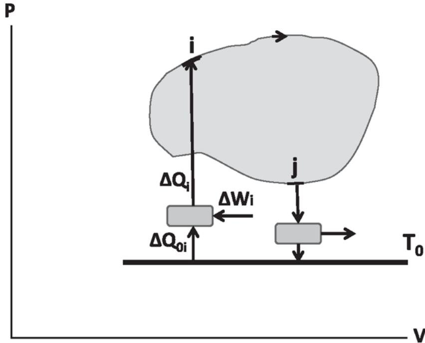
Figure 24.1 A system is taken quasi-statically through a cycle. In the segment labeled  $i$  it needs some heat  $\Delta Q_i$ , which it gets from a Carnot refrigerator operating between the system's current temperature and a reservoir at  $T_0$ . The refrigerator needs work  $\Delta W_i$ . If it happens that  $\Delta Q_i < 0$ , as is the case at point  $j$ , the heat will be sucked out of the system by a Carnot engine and dumped into the reservoir at  $T_0$ .
