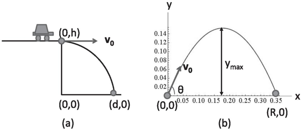
Figure 2.8 (a) A car flies off the cliff at  $(0, h)$  and lands at  $(d, 0)$ . (b) A projectile is launched with initial velocity  $\mathbf{v}_0 = (\mathbf{i} + \sqrt{3}\mathbf{j})\text{m/s}$ . The range is  $R = 0.35\text{ m}$  and the maximum height reached is  $y_{\text{max}} = 0.15\text{ m}$ .
