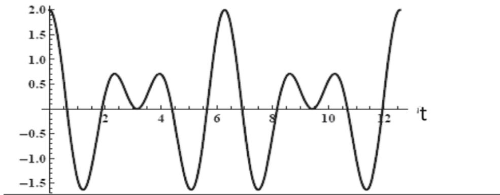
Figure 19.2 Superposition of two waves of unit amplitude  $A = 1$  and angular frequencies  $\omega_1 = 2$ , and  $\omega_2 = 3$ . At  $t = 0$  they are in step, at  $t = \pi$  their phases differ by  $\pi$  and they cancel, at  $t = 2\pi$  they are in step, and this repeats every  $2\pi$  seconds.
