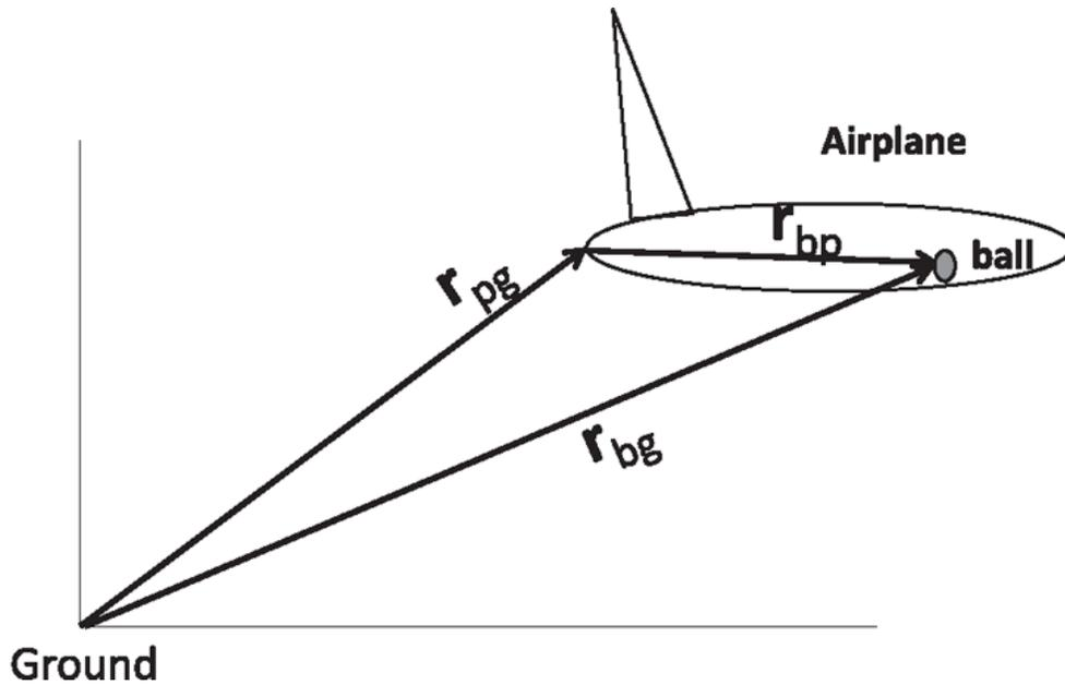
Figure 2.6 The position of the ball relative to (some origin on) the ground  $\mathbf{r}_{bg}$  is the vector sum of the position of the ball relative to the (tail of the) plane,  $\mathbf{r}_{bp}$ , and the position of (the tail of) the plane  $\mathbf{r}_{pg}$  relative to the ground.
