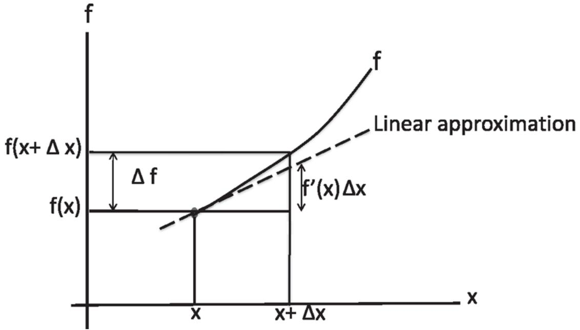
Figure 6.1 The change,  $\Delta f$ , in a function  $f(x)$  as  $x$  changes by  $\Delta x$ , may be approximated by  $\Delta f \approx f'(x)\Delta x$ , where  $f'(x) = \frac{df}{dx}$ . The solid line is the actual function and the dotted line is the approximation by a straight line of slope  $f'(x)$ .
