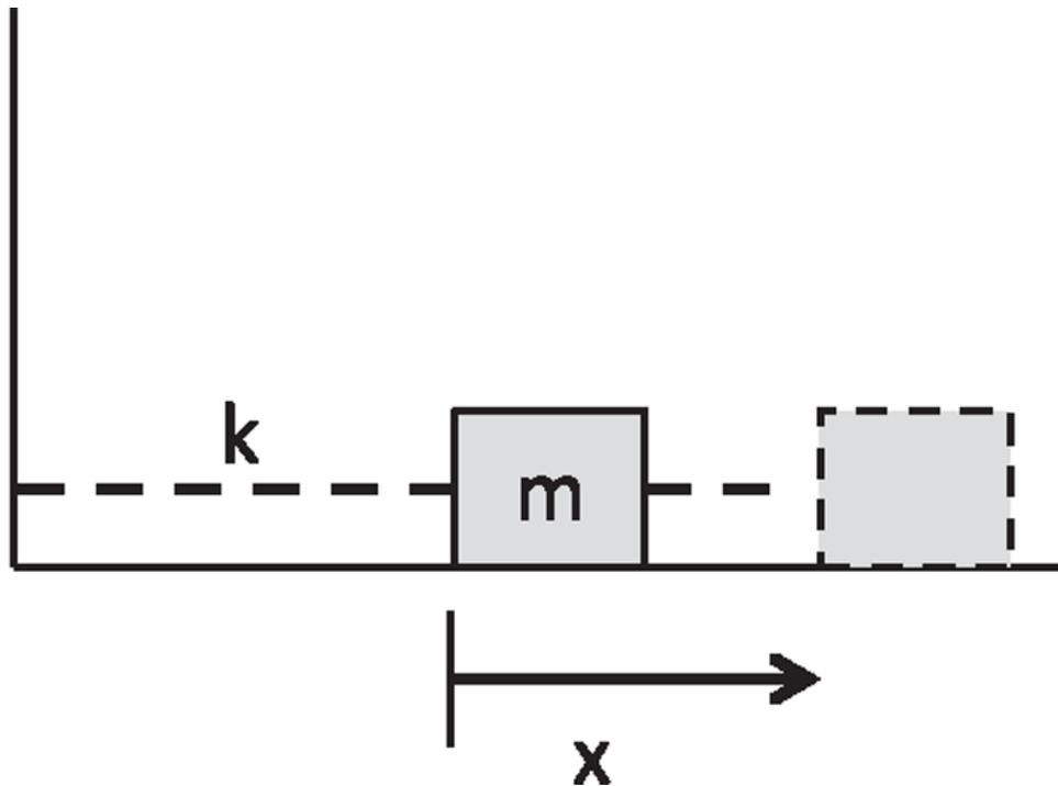
Figure 4.1 A mass  $m$  attached to a spring of force constant  $k$  in its equilibrium position, when the spring is neither extended nor compressed. The dotted outline of the mass shows it when it is displaced by an amount  $x$  from equilibrium.
