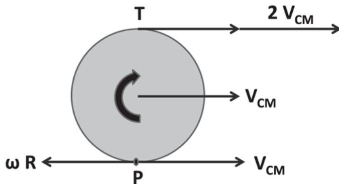
Figure 10.2 A tire of radius  $R$  that is rolling clockwise at  $\omega$  without slipping. At the contact point  $P$ , the CM velocity  $\mathbf{V}_{CM}$  cancels the tangential velocity  $\omega R$ , while at the top,  $T$ , it doubles it. The point  $P$  is instantaneously at rest with respect to the road.
