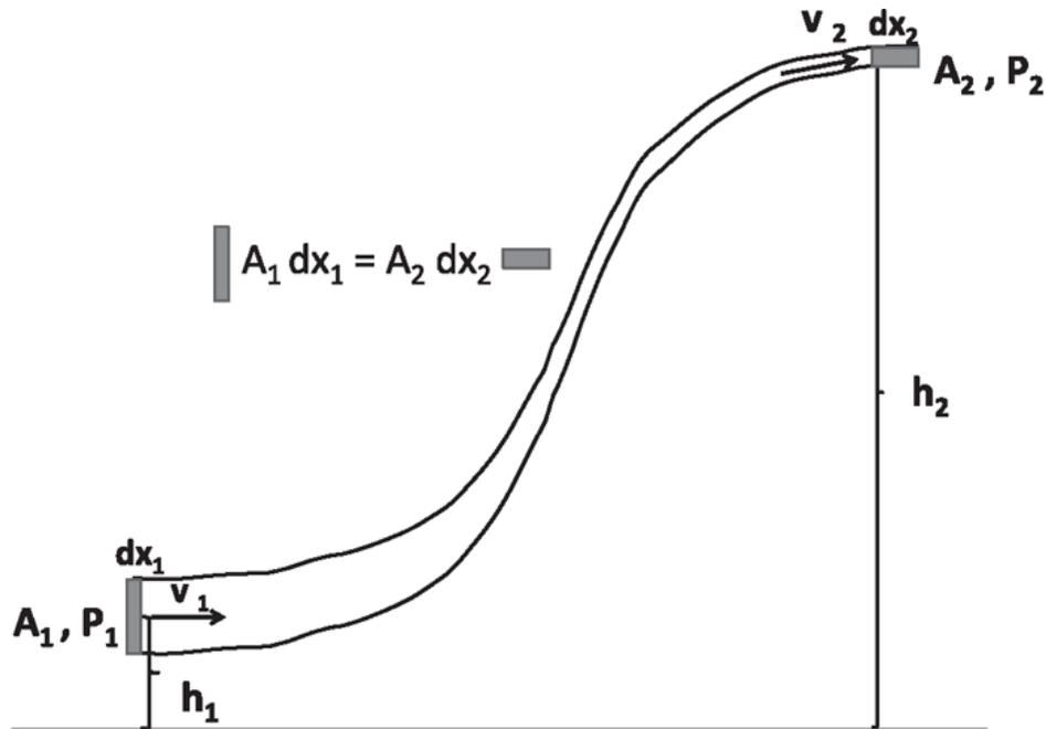
Figure 20.7 The flow of a fluid along a pipe of varying cross section, pressure, and height. We focus on the part initially between cross-sectional areas  $A_1$  and  $A_2$ . In a time  $dt$ , it is left unchanged but for a sliver of volume  $A_1 dx_1 = A_1 v_1 dt$ , which has been removed from the left and appended to the right end as a sliver of equal volume  $A_2 dx_2 = A_2 v_2 dt$ .
