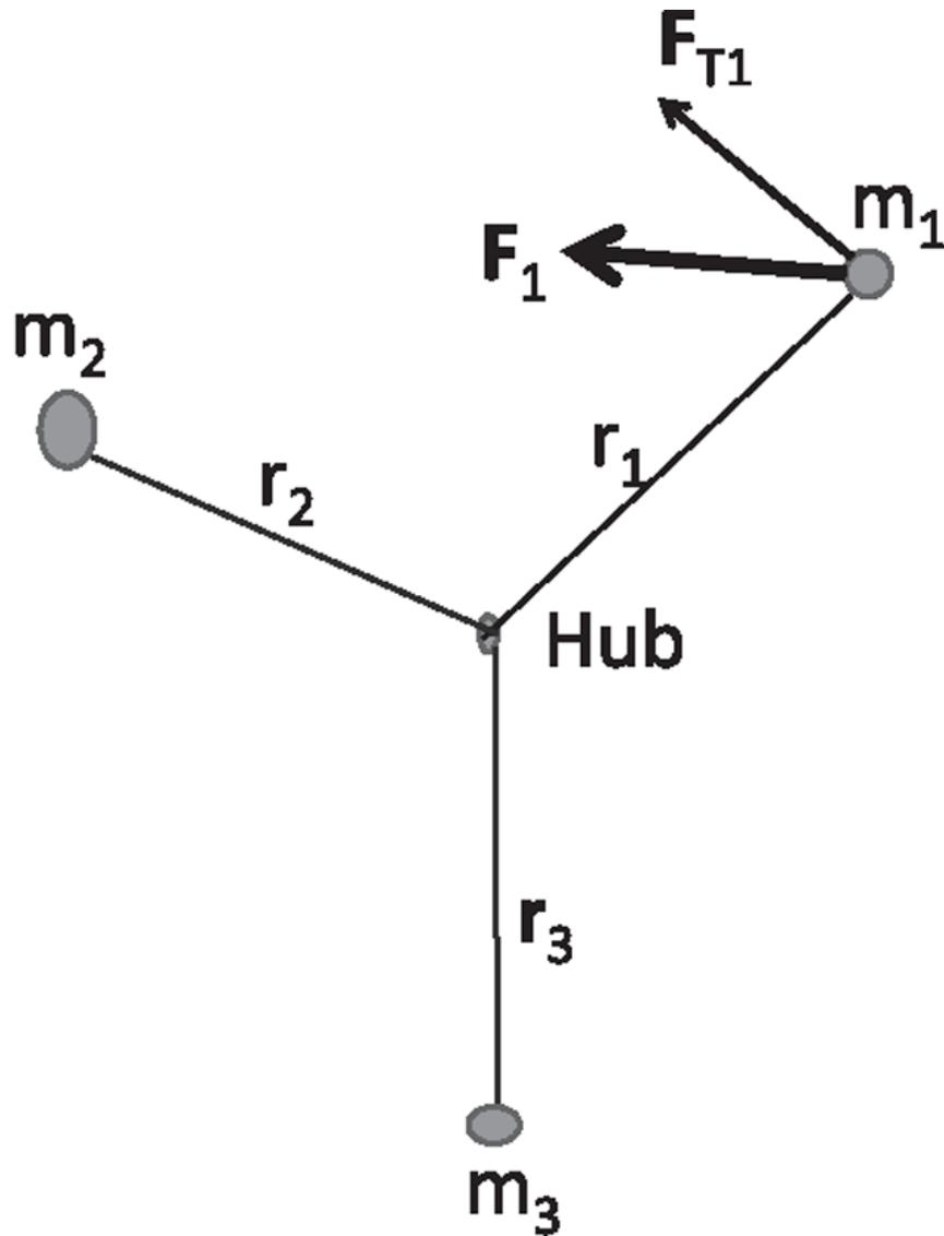
Figure 9.3 A simple rigid body made of three point masses attached to a fixed hub by three massless rigid rods. When a force  $F_1$  acts on 1, only the tangential component  $F_{T1}$  produces angular acceleration.
