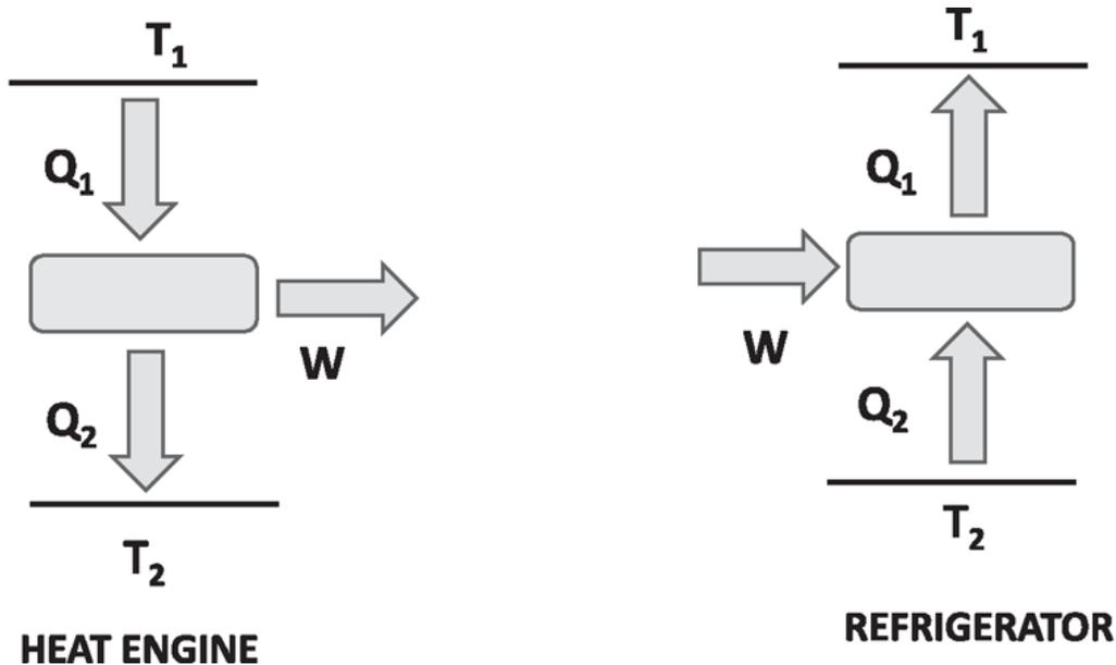
Figure 23.3 A heat engine (left) takes in heat  $Q_1$  from a reservoir at  $T_1$ , does some work  $W$ , and rejects heat  $Q_2$  to a colder reservoir at  $T_2$ . Things go the other way in a refrigerator (right): work  $W$  is pumped in to transfer heat  $Q_2$  from  $T_2$  to a higher temperature  $T_1$ .
