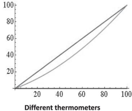
Figure 21.2 The  $x$ -axis is labeled by the reading of a reference thermometer, say with mercury. Along the  $y$ -axis are plotted the readings as per another—say, an alcohol—thermometer (curved line) along with a straight line  $y = x$ , which is just the reading of the same mercury thermometer plotted for easy comparison.
