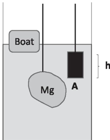
Figure 20.6 The irregular object of mass  $M$  displaces a volume of liquid equal to its own. The loss in its weight is the weight of that body of liquid. This is more readily seen for a regular object like the cylinder shown to the right. At the top left is a boat whose weight equals the weight of the liquid displaced by the fraction immersed.
