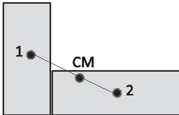
Figure 8.3 (Top) A rod of length  $L$  and mass  $M$ . (Bottom) An L-shaped object made of two rectangles. The points 1 and 2 are the CMs where all their mass may be assumed to be concentrated. The point marked CM is the weighted sum of 1 and 2.
