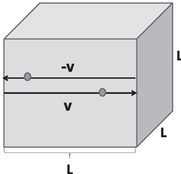
Figure 22.1 A cubic box with  $N$  gas atoms inside. The figure shows an atom of velocity  $v$  hitting the shaded wall and reversing its velocity. The corresponding momentum change is due to the wall, which exerts a force on the atom. The opposite force the atom exerts on the wall is its contribution to the pressure.
