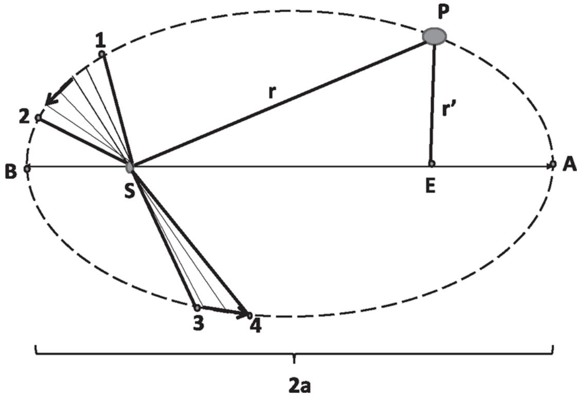
Figure 7.1 The solar system seen from afar, with just one planet  $P$  shown. The orbit is an ellipse with the sun  $S$  at one focal point, and a major axis  $2a$  that obeys  $r + r' = 2a$ . The position vector sweeps out equal areas in equal times, for example, between 1 and 2 and between 3 and 4.
