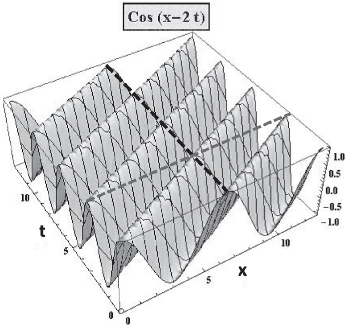
Figure 18.4 The wave  $A \cos(kx - \omega t)$  with  $A = 1$ ,  $k = 1$ ,  $\omega = 2$  or  $\lambda = 2\pi$ ,  $T = \pi$  in the range  $[0, 4\pi]$  for both  $x$  and  $t$ . If you slice it at fixed  $t$ , you will see two full periods in  $x$  (see dotted line at  $t = 2\pi$ ), and if you slice it at fixed  $x$ , you will see four periods in  $t$  (see dotted line at  $x = 2\pi$ ). The lines track the maxima or crests, but one could pick any point within the cycle.
