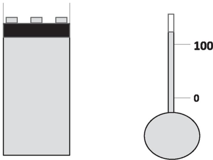
Figure 21.1 Left: The gas is inside the cylinder capped by a piston of area  $A$ . The weights on the piston exert a force  $F$  and pressure  $\frac{F}{A}$ . Right: A thermometer with a liquid that expands from the bulb into the thin calibrated stem.
