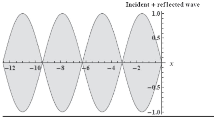
Figure 19.7 Nodes and anti-nodes on a string with  $A = 0.5$  and  $k = 1$  or  $\lambda = 2\pi$ . The incoming and reflected waves form a *standing wave*, with nodes at  $0, -\pi, -2\pi, \dots$  and anti-nodes at  $-\frac{\pi}{2}, -\frac{3\pi}{2}, \dots$ . The vibrating string is a blur, shown by the shaded region.
