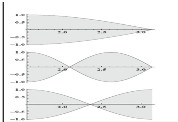
Figure 19.9 From the top: First two modes of vibration of a tube of length  $\pi$  closed at the right end and open at the left end followed by the first mode of a tube of length  $\pi$  open at both ends. You can read off the  $\lambda$ 's by inspection and deduce the frequencies from  $v = \lambda f$ .
