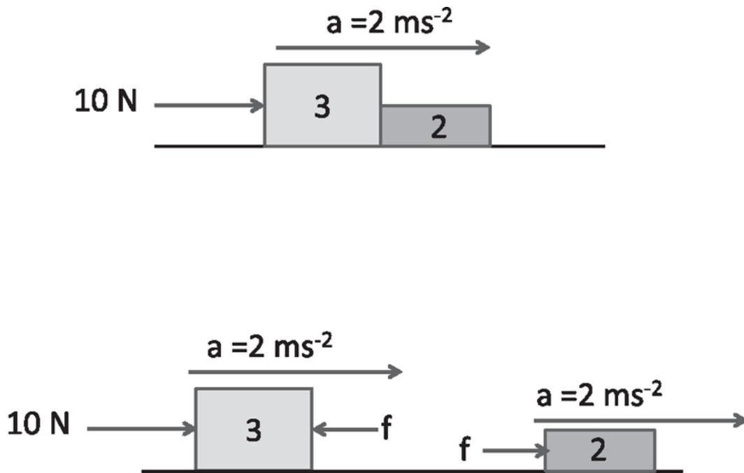
Figure 3.3 Top: A force of 10 N acts on the two blocks, viewed as a single entity. Bottom: The free-body diagram for the two blocks showing all the forces *on* each block. Notice the third law is being invoked.
