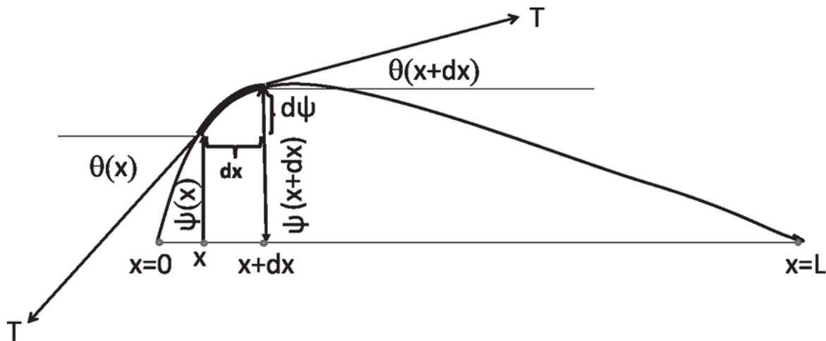
Figure 18.2 The string under tension  $T$  has mass  $\mu$  per unit length and is fixed at  $x = 0$  and  $x = L$ . The highlighted segment has a width  $dx$ , with the same tension  $T$  pulling the two ends but at slightly different angles. The displacement  $\psi$  and angles  $\theta$  are exaggerated for clarity. The derivation is valid only when all these are very small.
