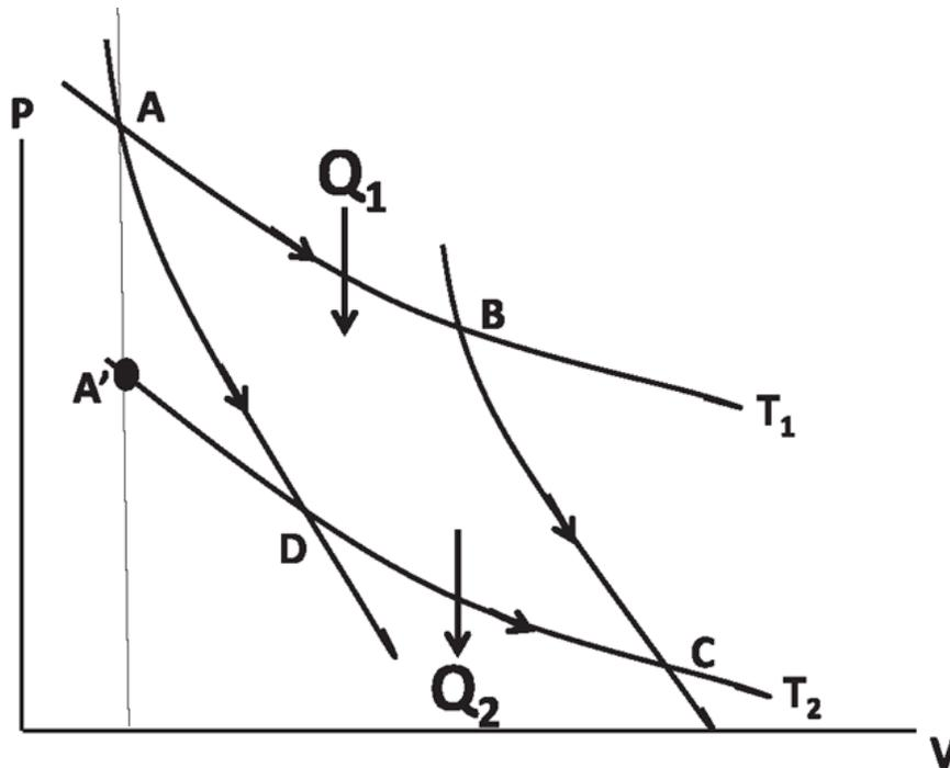
Figure 23.2 The figure shows two isothermal curves at  $T_1$  and  $T_2$  and two adiabatic curves crossing them. In the latter case  $P$  falls more rapidly with increasing  $V$  because it gets no help from outside.
