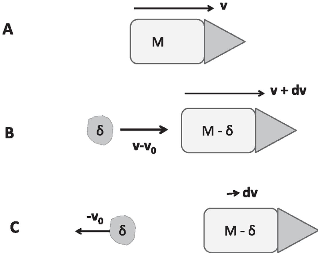
Figure 8.7 (A) The rocket at time  $t$  as seen from the ground. (B) The rocket at time  $t + dt$  as seen from the ground. It has lost mass  $\delta$  in the form of emitted gases and gained speed  $dv$ . The fumes of mass  $\delta$  (the blob) are moving at a speed  $(v - v_0)$  relative to the ground. (C) The rocket and fumes at time  $t + dt$  in the frame moving at velocity  $v(t)$ . The fumes have an exhaust velocity  $-v_0$  in the rocket frame.
