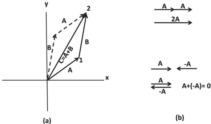
Figure 2.2 Adding vectors. Part (a) shows how to add vectors and that  $\mathbf{A} + \mathbf{B} = \mathbf{B} + \mathbf{A}$ . Part (b) illustrates the meaning of multiplying a vector by a number (2 in this example) and the null vector  $\mathbf{0}$ .
