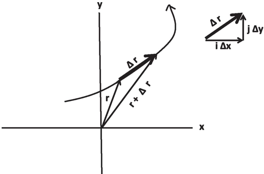
Figure 2.5 The particle moving along some curved path goes from  $\mathbf{r}$  at time  $t$  to  $\mathbf{r} + \Delta\mathbf{r}$  at time  $t + \Delta t$ . The velocity  $\mathbf{v}$  is the limit of the ratio  $\frac{\Delta\mathbf{r}}{\Delta t}$  as  $\Delta t \rightarrow 0$ , and thus parallel to  $\Delta\mathbf{r}$ , which eventually becomes tangential to the curve.
