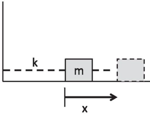
Figure 17.1 The mass  $m$  rests on a table and is connected to a spring of force constant  $k$ , which is anchored to the wall. The displacement from equilibrium is denoted by  $x$ . It is positive in the figure but it could also be negative if the mass were to be displaced the other way.
