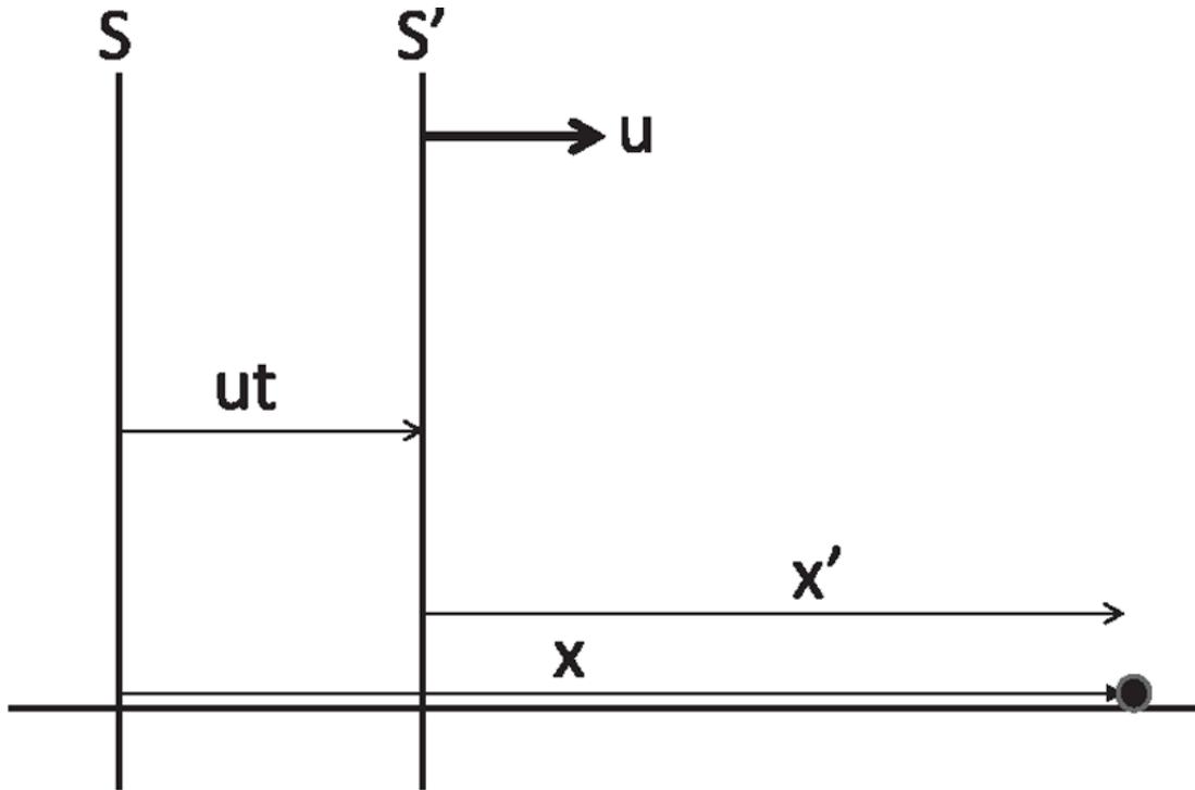
Figure 12.1 The same event (solid dot) is assigned coordinates  $(x,t)$  by me (S) and  $(x',t')$  by you (S'). In the pre-Einstein days  $t = t'$  not only initially (when our origins crossed and clocks were synchronized) but always. At time  $t$ , your origin is to the right of mine by an amount  $ut$ . So the firecracker going off at location  $x$  at time  $t$  according to me happens at  $x' = x - ut$  according to you.
