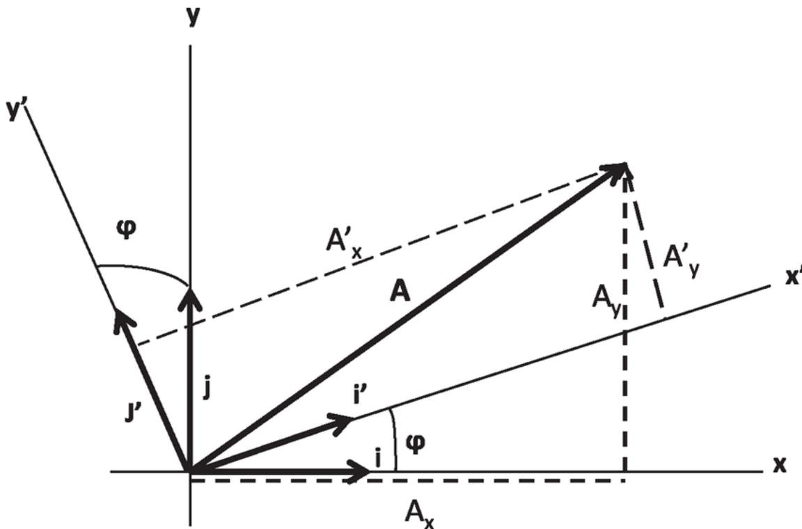
Figure 2.4 The same vector  $\mathbf{A}$  is written as  $\mathbf{i}A_x + \mathbf{j}A_y$  in one frame and as  $\mathbf{i}'A'_x + \mathbf{j}'A'_y$  in the other. The dotted lines indicate the components in the two frames.
