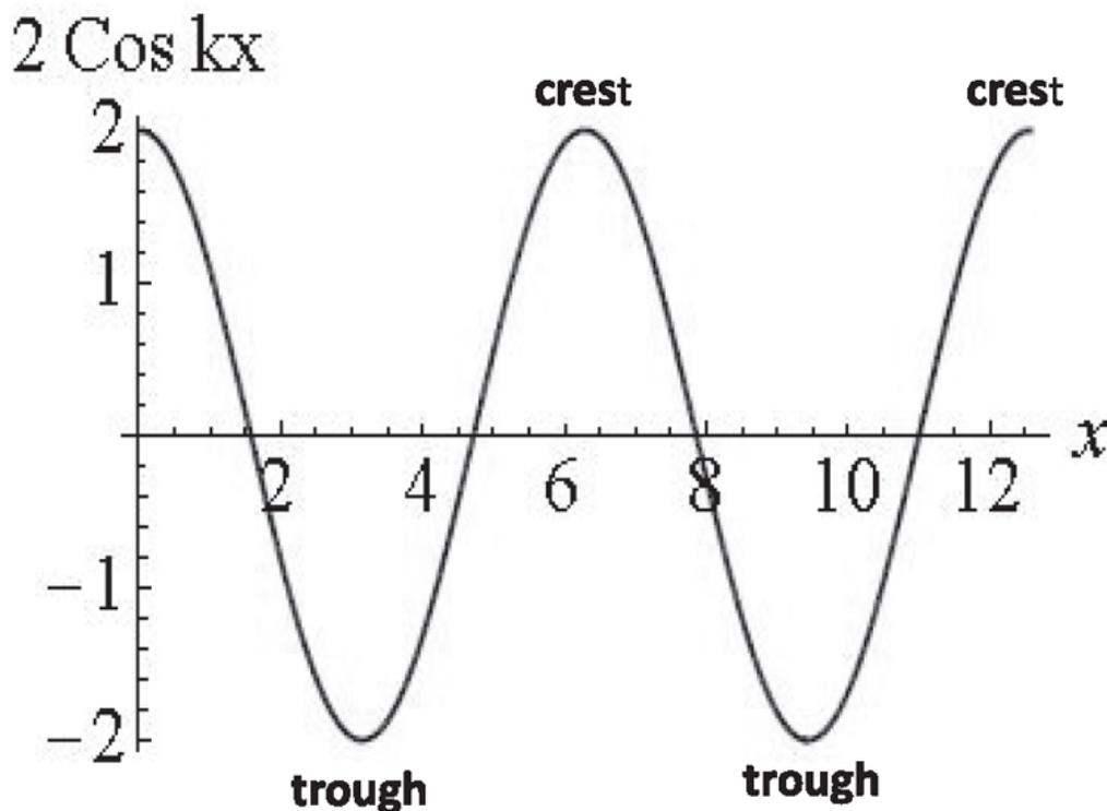
Figure 18.3 The wave  $A \cos(kx - \omega t)$  at  $t = 0$  as a function of  $x$  for the choice  $A = 2$ ,  $k = 1$ . For  $k = 1$ ,  $\lambda$  should be  $2\pi \approx 6.28$  according to Eqn. 18.29, and indeed it is. The maxima are called *crests* and the minima are called *troughs*.
