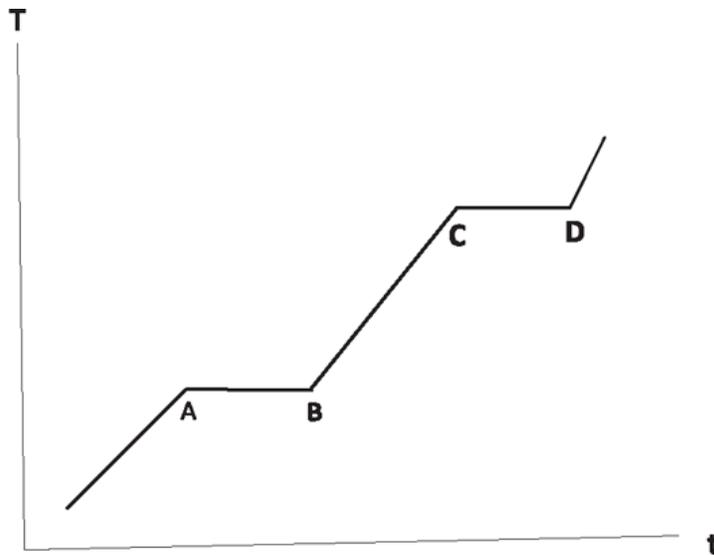
Figure 21.5 Different phases of water from ice below  $0^\circ\text{C}$  to water above  $100^\circ\text{C}$ . As time  $t$  increases, a steady flow of calories first heats the ice below  $0^\circ\text{C}$  to A, where it melts at  $0^\circ\text{C}$  between A and B. The water then heats up between B and C, and then it evaporates at  $100^\circ\text{C}$  between C and D, before becoming superheated steam.
