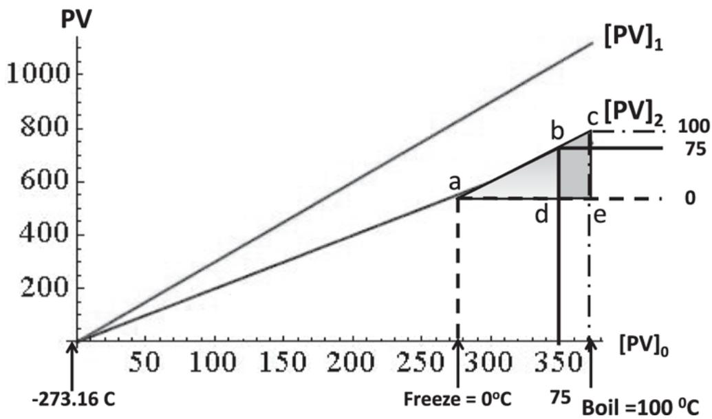
Figure 21.3 Comparison of different gas thermometers labeled 0, 1, and 2. The  $x$ -axis is labeled by one and the other two correspond to two other gas thermometers, possibly filled with different dilute gases. The linearity of the graphs guarantees that the thermometers will agree not only at 0 and 100, where they have to, but also everywhere in between given the similarity of triangles  $abd$  and  $ace$ . When  $[PV]_0 = 350$ , the temperature is  $75^\circ\text{C}$ .
