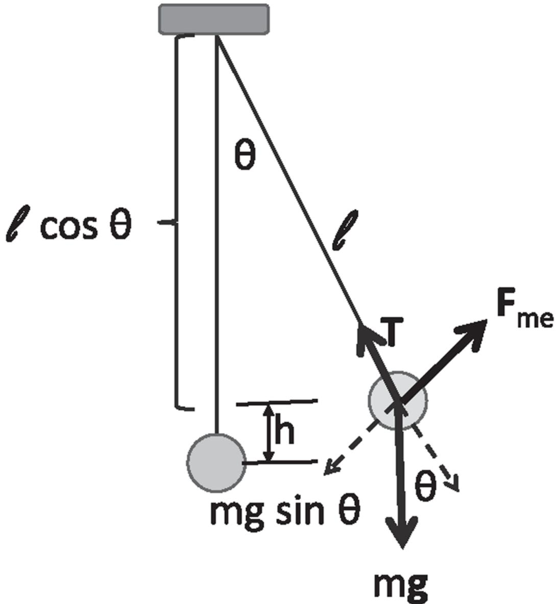
Figure 9.5 A pendulum made up of a massless string length  $l$  and a bob of mass  $m$ . The force  $mg$  is resolved in the radial and tangential directions. The bob has climbed up a height  $h = l - l \cos \theta$ .
