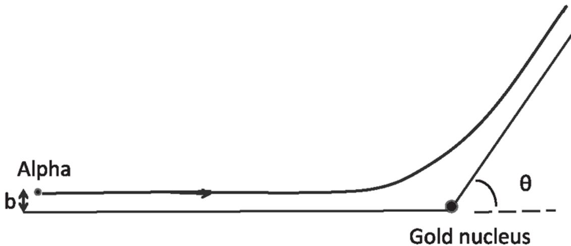
Figure 8.10 An alpha particle approaching a gold nucleus with impact parameter  $b$ . If you assume the nucleus is immobile and exerts a Coulomb force  $1/r^2$ , you can calculate the direction  $\theta$  in which the alpha particle will emerge, as a function of  $b$  and the energy. If a beam of particles with a distribution of  $b$ 's is given, one can predict the particle flux in any direction  $\theta$ .
