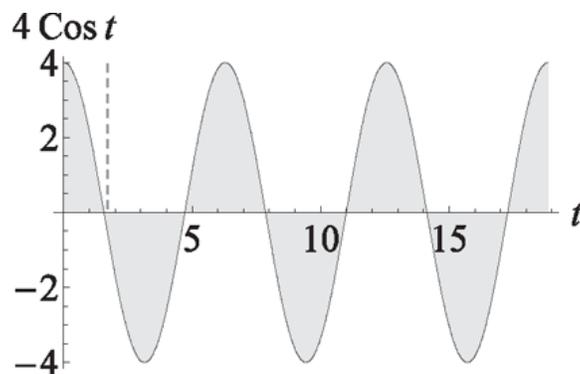
Figure 17.2 The function  $A \cos \omega t$  for the case  $A = 4$ ,  $\omega = 1$ . The dotted vertical line is another possible way to set the clock to zero, another choice of phase, namely  $\phi = \frac{\pi}{2}$ .
