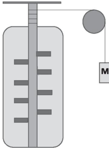
Figure 21.7 Joule's experiment to find the mechanical equivalent of heat,  $4.2\text{kJ/kcal}$ . As the weight descends, the fins turn and heat up the water. The missing mechanical energy in the weight becomes heat energy. (It is assumed that the rest of the apparatus does not absorb any appreciable part of the generated heat.)
