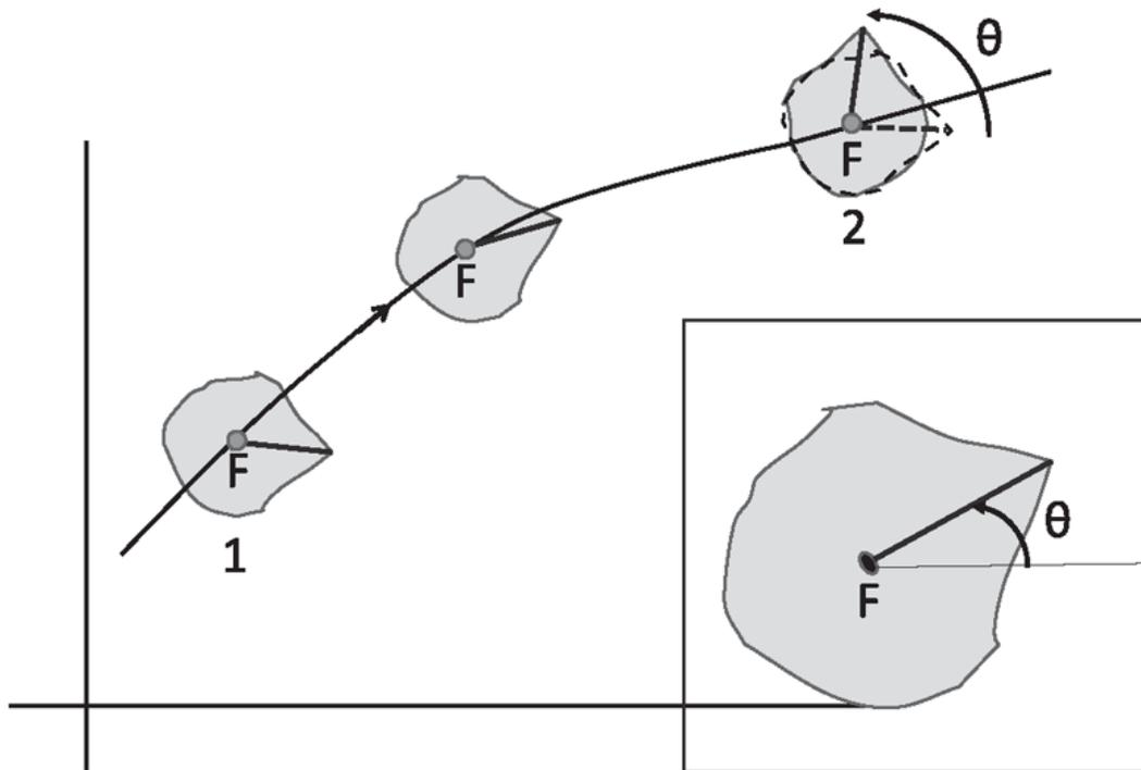
Figure 9.1 A rigid planar body undergoing translation and rotation in a plane as it goes from state 1 to state 2. The dot represents the fixed point  $F$ . The solid line from the  $F$  to the pointy edge of the object allows us to follow its rotation. In state 2 the original orientation is shown in dotted lines and the curved arrow shows the rotation  $\theta$  needed to bring it to the final orientation.
