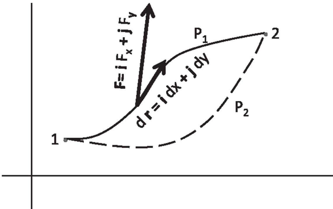
Figure 6.3 The line integral of a force between points 1 and 2 along a path  $P_1$  is the sum of dot products  $\mathbf{F} \cdot d\mathbf{r}$  over tiny segments that make up the path, in the limit  $d\mathbf{r} \rightarrow \mathbf{0}$ . Also shown by a dotted line is another path  $P_2$  between the same end points.
