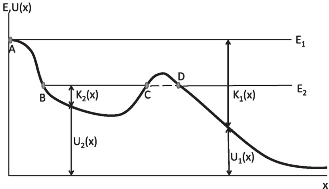
Figure 6.5 The roller-coaster ride. The total energy is fixed at  $E_1$  or  $E_2$  in the two examples discussed. At every point  $x$ , the sum of the potential energy  $U(x)$  and the kinetic energy  $K(x)$  equals a constant  $E$ . If the energy is  $E_2$ , the coaster can only be found between  $B$  and  $C$  or to the right of  $D$ . It is disallowed in the region  $CD$  where the potential energy exceeds the total energy, and  $K$  would have to be negative.
