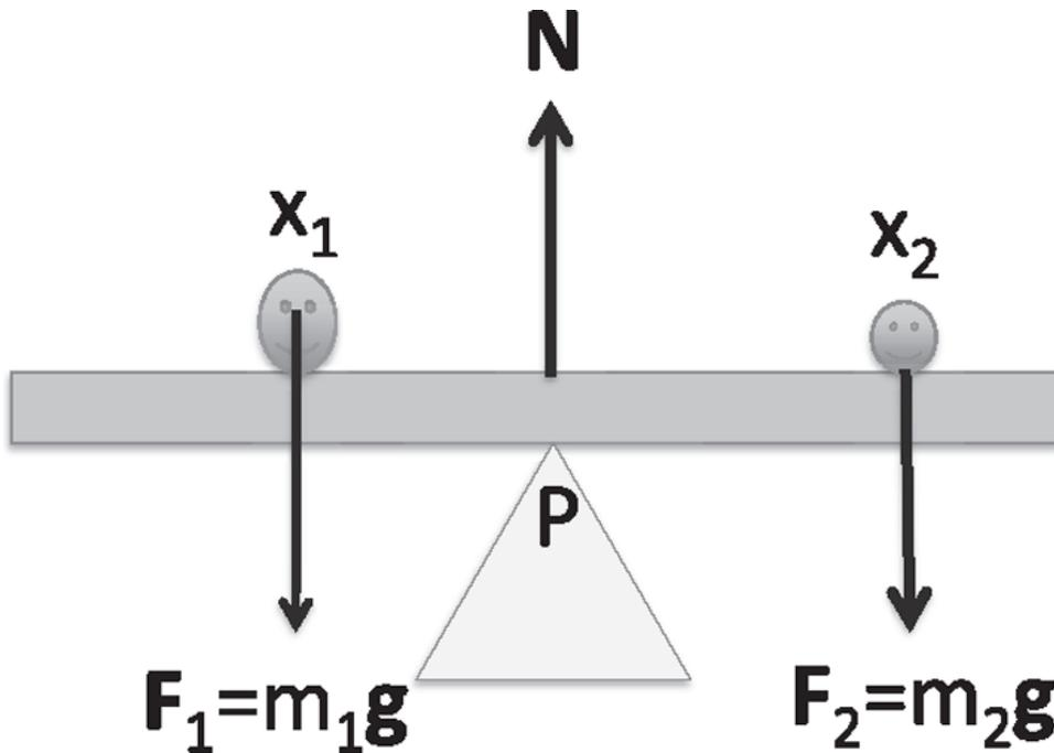
Figure 11.1 Two kids on a seesaw. The supporting pivot provides a force  $\mathbf{N}$  upward. The total torque due to the kids' weights  $\mathbf{F}_1 = m_1\mathbf{g}$ ,  $\mathbf{F}_2 = m_2\mathbf{g}$  and the pivot force  $\mathbf{N}$  is zero.
