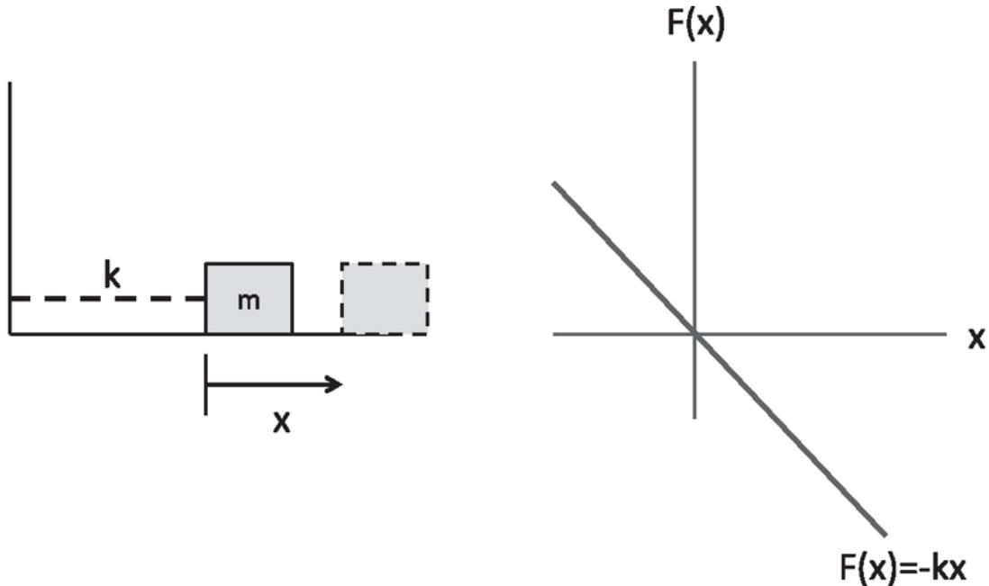
Figure 3.1 (Left) The mass  $m$  is attached to a spring (dotted line) of force constant  $k$ . The other end of the spring is attached to a wall. The displacement  $x$  is measured from the equilibrium position of the spring. (Right) The force  $F(x)$  as a function of  $x$ .
