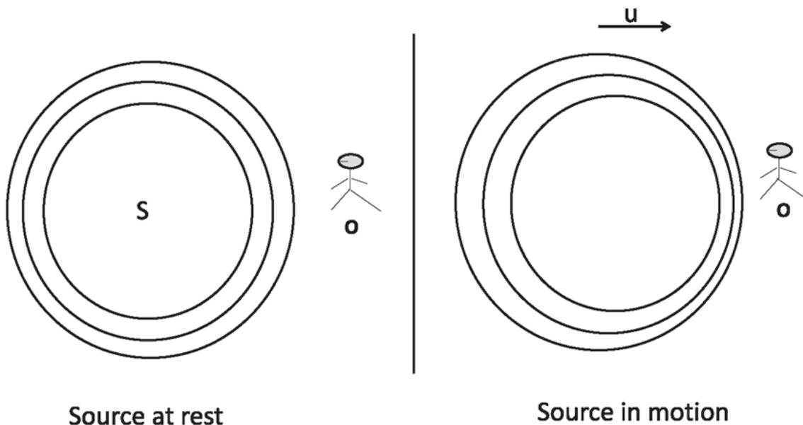
Figure 19.1 At the left we have a source at rest and observer  $O$  at rest. The three crests emitted are equally spaced in the air and also as perceived by  $O$ . At the right we have the source moving at velocity  $u$ . The wavefronts now get crunched in the forward direction because the source travels a bit to the right between emitting one crest and the next. In the backward direction the opposite happens.
