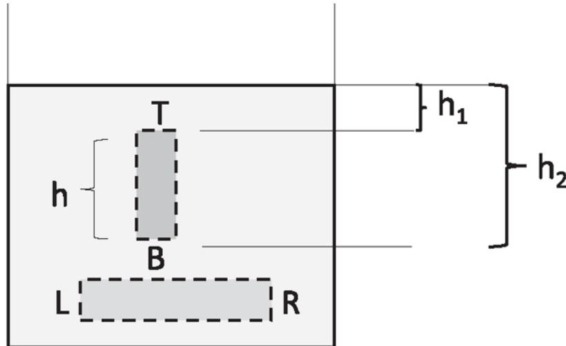
Figure 20.2 The horizontal dotted cylinder marks a part of the fluid in equilibrium under forces from the left  $L$  and right  $R$ . The vertical dotted cylinder marks a part of the fluid in equilibrium under forces from the top  $T$  and bottom  $B$  and its weight  $Mg$ .
