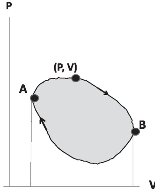
Figure 23.1 The work done by a gas as it goes over a closed cycle equals the area enclosed by the cycle in the  $P - V$  plane. During  $AB$  the gas expands and does work, and during  $BA$  it is compressed and has work done on it. The shaded area is the algebraic sum of the two.
