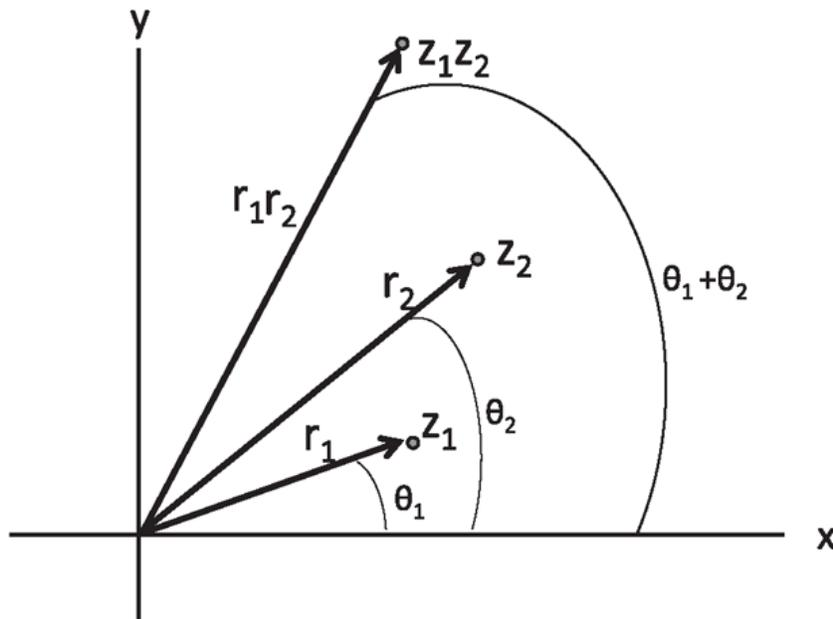
Figure 16.3 The rule for multiplying  $z_1$  and  $z_2$ : add the phase angles  $\theta_1$  and  $\theta_2$  to get the phase of the product and multiply the amplitudes  $r_1$  and  $r_2$  to get the amplitude of the product.
