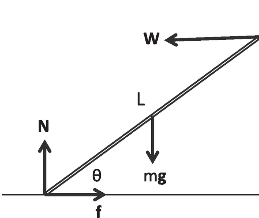
Figure 11.3 A ladder of mass  $m$  and length  $L$  is leaning against a frictionless wall and standing on a floor with some coefficient of friction  $\mu_s$ . The normal and frictional forces due to the floor are shown separately.
