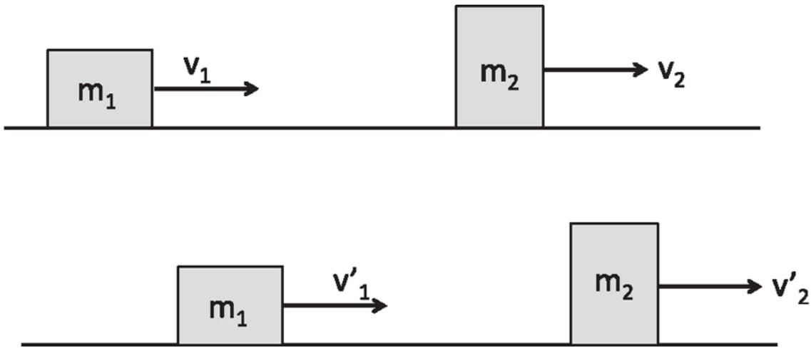
Figure 8.8 (Top) A body of mass  $m_1$  and velocity  $v_1$  collides with a body of mass  $m_2$  and velocity  $v_2$ , with all velocities shown as positive. (Bottom) The two bodies with final velocities  $v'_1$  and  $v'_2$ .
