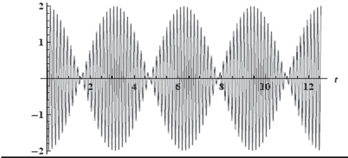
Figure 19.3 Beats due to two waves of unit amplitude  $A = 1$  and large but nearly equal angular frequencies  $\omega_1 = 41$ ,  $\omega_2 = 39$ . The (angular) beat frequency is supposed to be  $\omega_b = 41 - 39$  rads/s, which means a time  $T = \frac{2\pi}{\omega_b} = \pi$  between beats, in accord with the figure.
