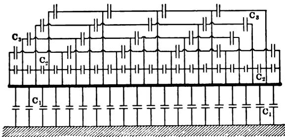
Fig. 89. Distributed capacity of a high-potential transformer coil.
