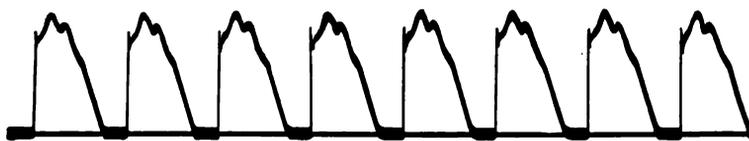
Fig. 71. Unidirectional e.m.f. produced between rectifier neutral and transformer neutral.
