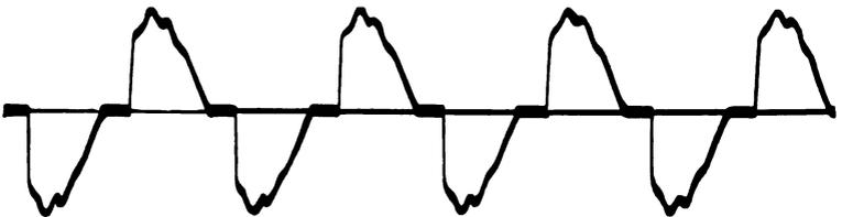
Fig. 70. Alternating e.m.f. impressed upon rectifier tube.
