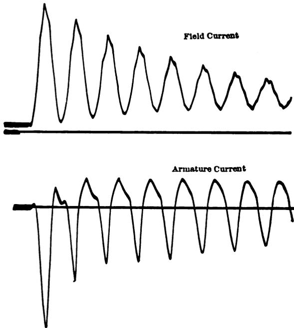
Fig. 51. Three-phase short-circuit current of a turbo-alternator.
