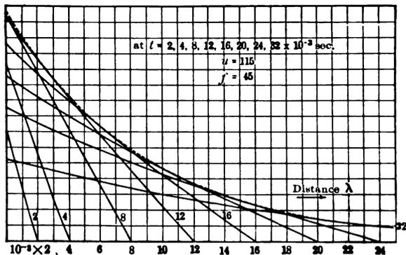
Fig. 99. Spread of amplitude of electric traveling wave.
