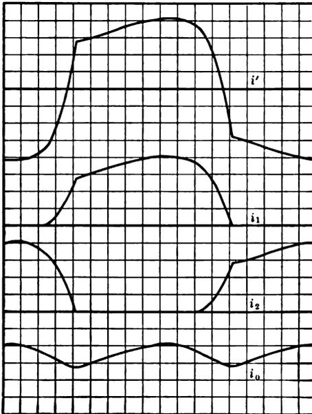
Fig. 65. Current waves of constant-current mercury arc rectifier.
