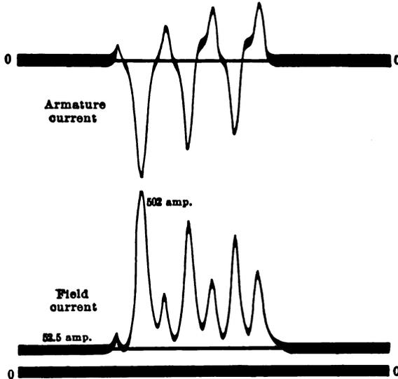
Fig. 53. Single-phase short-circuit current of a three-phase turbo-alternator.
