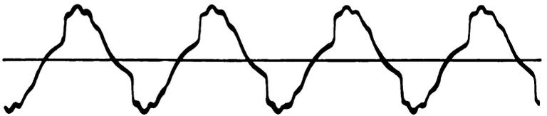
Fig. 68. Secondary terminal e.m.f. of transformer.
