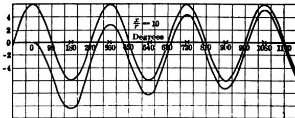
Fig. 8. Starting current of an inductive circuit.
