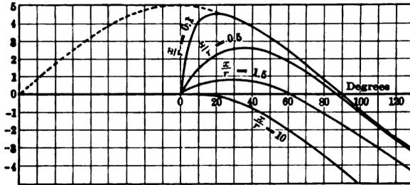
•Fig. 7. Starting current of an inductive circuit.
