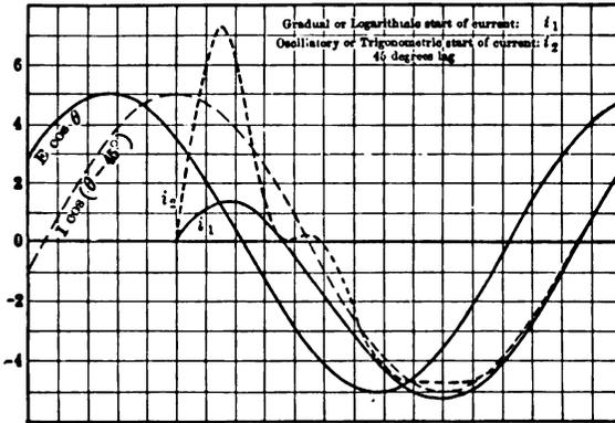
Fig. 4. Starting of an alternating-current circuit having inductance.
