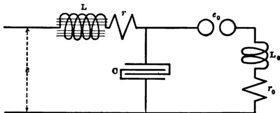
Fig. 16. Oscillating-current generator.
