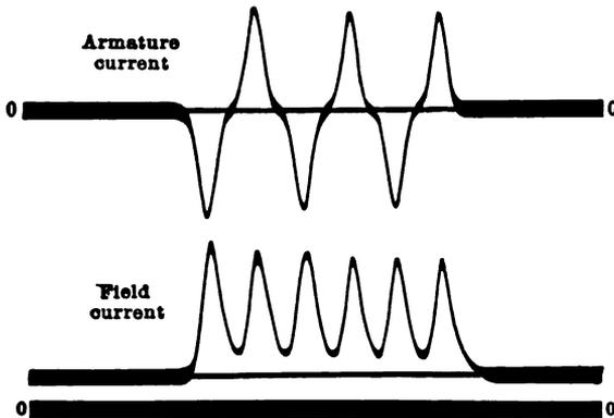
Fig. 52. Single-phase short-circuit current of a three-phase turbo-alternator.
