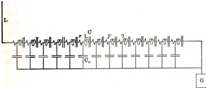
Fig. 91. Equivalent circuit of a multi-gap lightning arrester.
