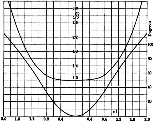
Fig. 98. Alternating magnetic flux distribution in solid iron.
