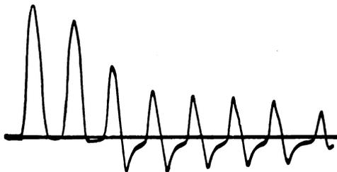
Fig. 47. Starting current of a 25-cycle transformer.
