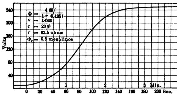
Fig. 6. Building-up curve of a shunt generator.
