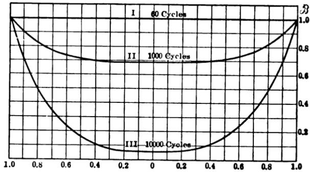
Fig. 95. Alternating magnetic flux distribution in solid iron.
