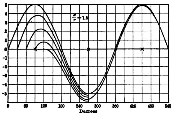
Fig. 9. Starting current of an inductive circuit.
