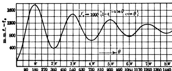
Fig. 49. Transient term of polyphase magnetomotive force.
