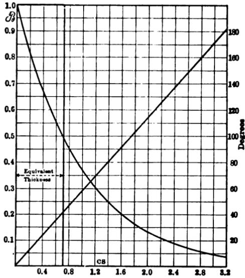
Fig. 94. Alternating magnetic flux distribution in solid iron.
