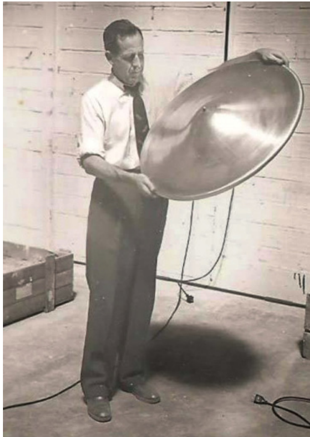
Inspecting one of the solid aluminum ‘ballistic electrode’ discs used in experiments at the Bahnson labs ca. 1957
