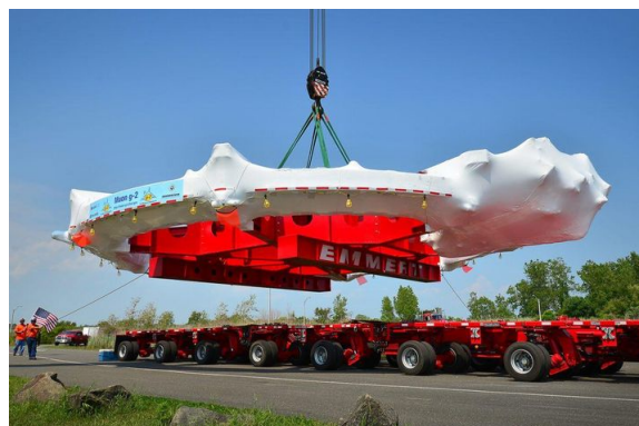
Fig. 9: Transportation of the 600 ton magnet to Fermilab
