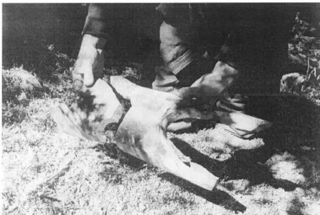
Portion of eight-foot long Triatic Insulator (Marconi period) found in dump
