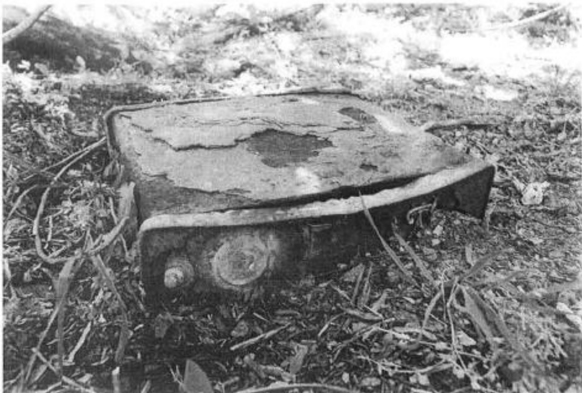
1928 condenser unit (originally was oil-filled) left in Marconi dump
