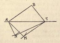
ordinary ray will be the tangent-plane to the sphere through the line whose trace is T, while the wave-front corresponding to the extraordinary ray will be the tangent-plane to the spheroid through the same line. The points of contact N
