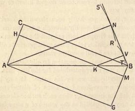
Huygens' principle the secondary wave from A is at the instant t a sphere RNS of radius equal to AG: the disturbance from H, after meeting the interface at K, will generate a secondary wave TV of radius equal to KM, and similarly the secondary wave corresponding to any other element of the original wave-
