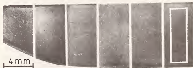
FIGURE 1. Moiré topogram of the x-ray interferometer (for details see Ref. [3], p. 31). As can be recognized, the lattice spacing varies by less than 4 \times 10^{-8} in the given material. The region used in the experiments is marked.
