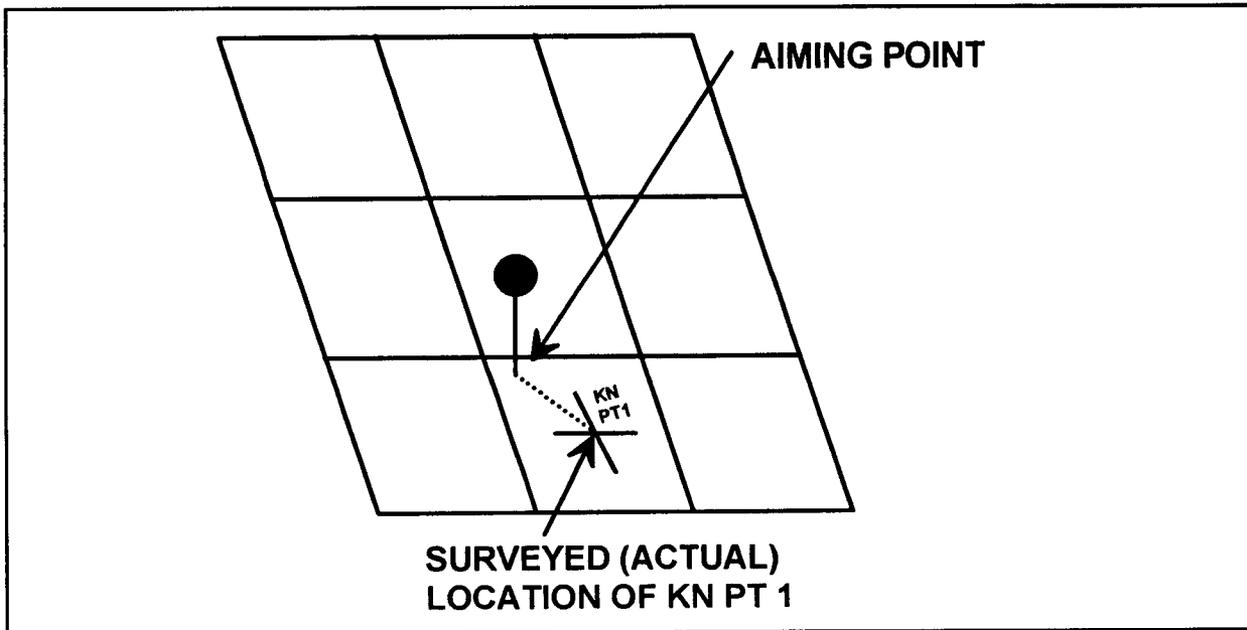
**Figure 10-2. Difference Between Aiming Point and Surveyed Location.**
