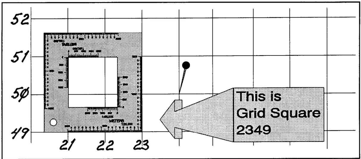
Figure 6-7. Position Plotted in Grid Square 2349.
