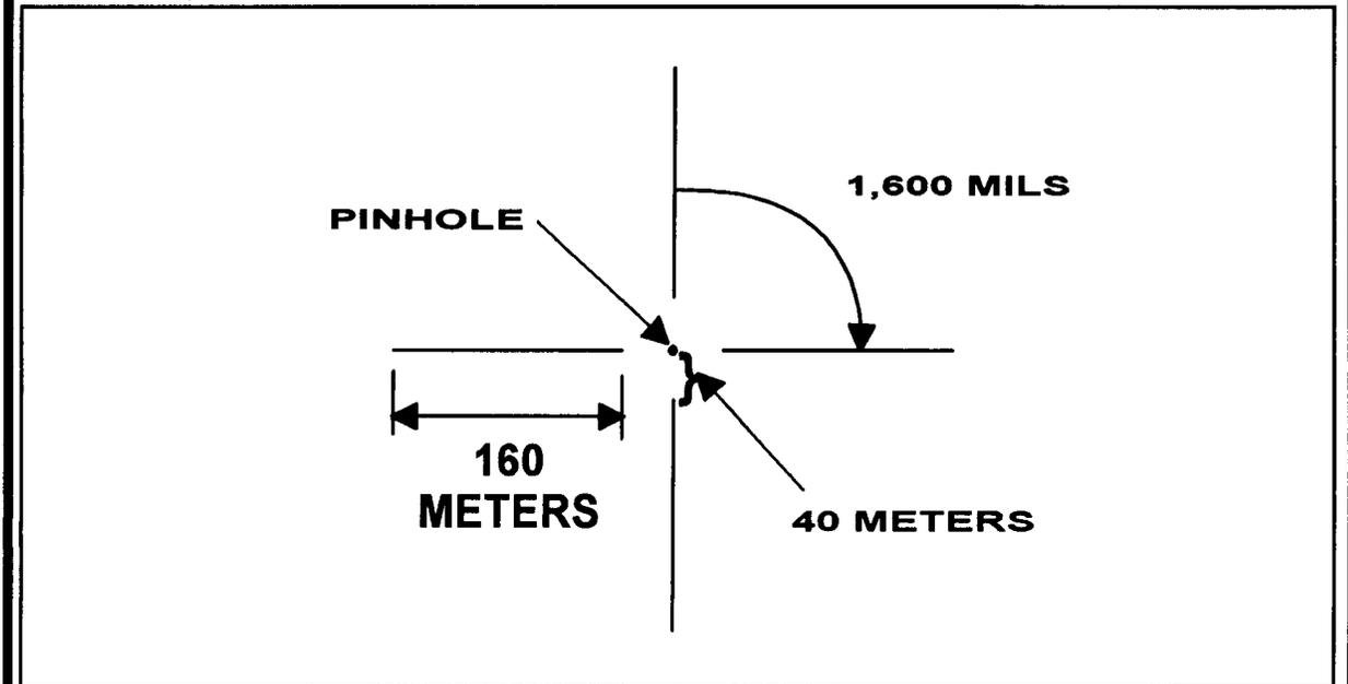
**Figure 6-10. Dimensions of a Completed Tick Mark.**
