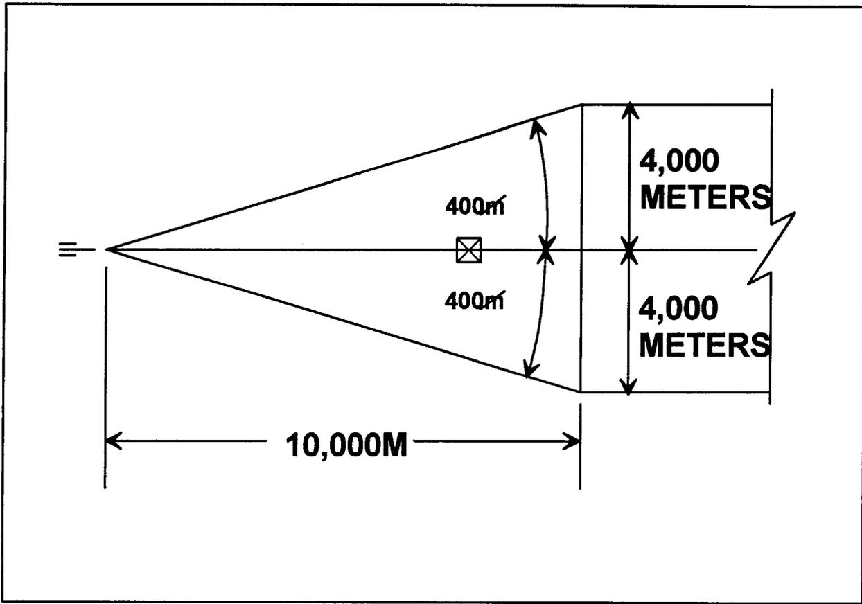
**Figure 10-25. Deflection Transfer Limits--Ranges Greater Than 10,000 Meters.**
