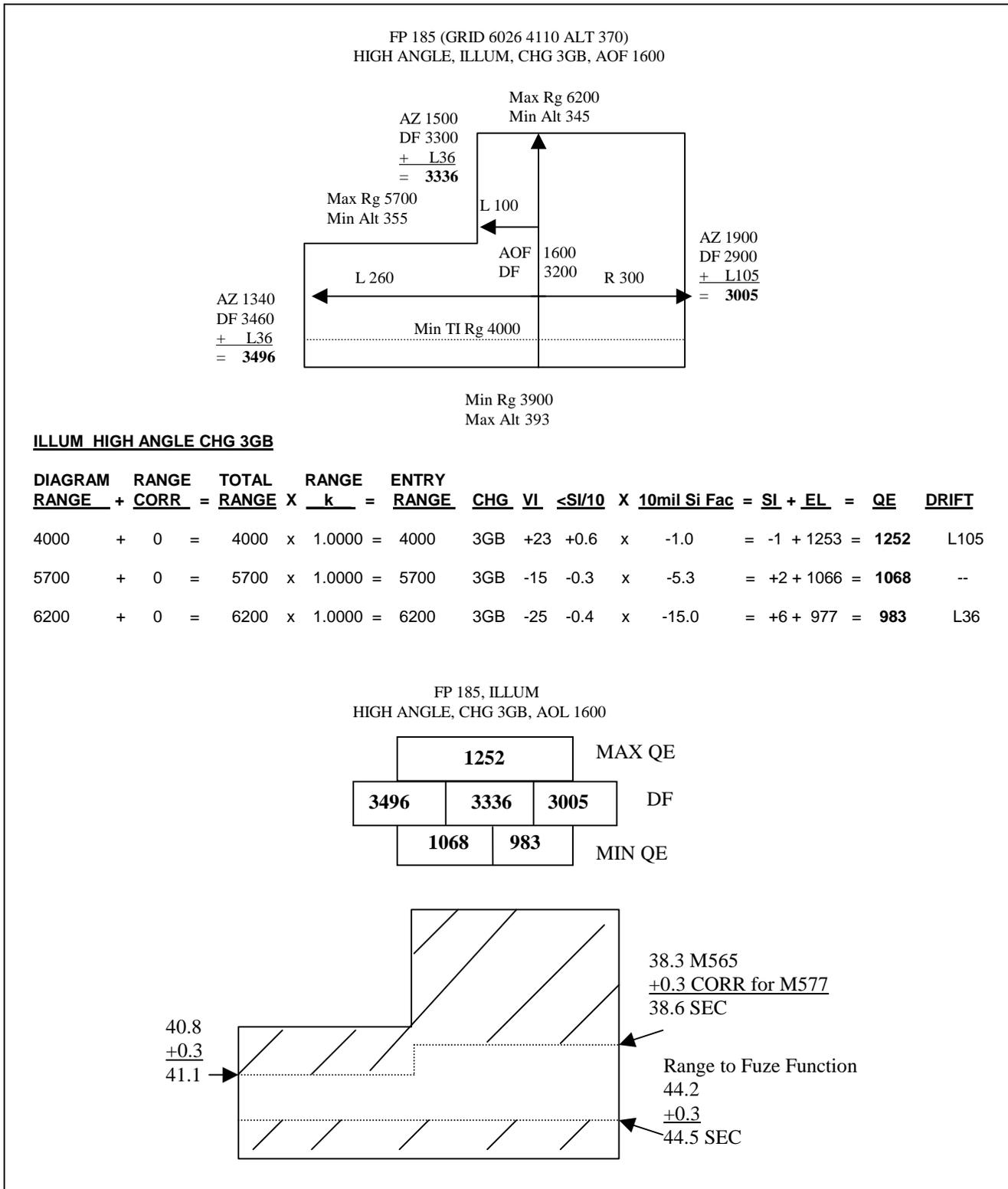
Figure 15-15. Example of High Angle Safety, Shell Illum
