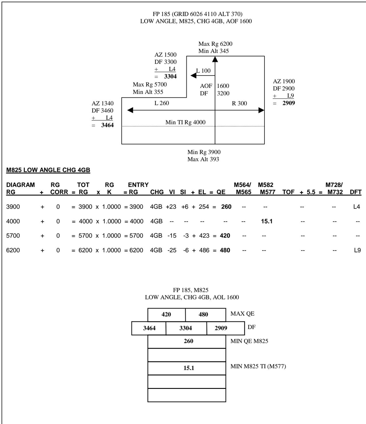
Figure 15-7. Example of Low Angle Safety Shell M825
