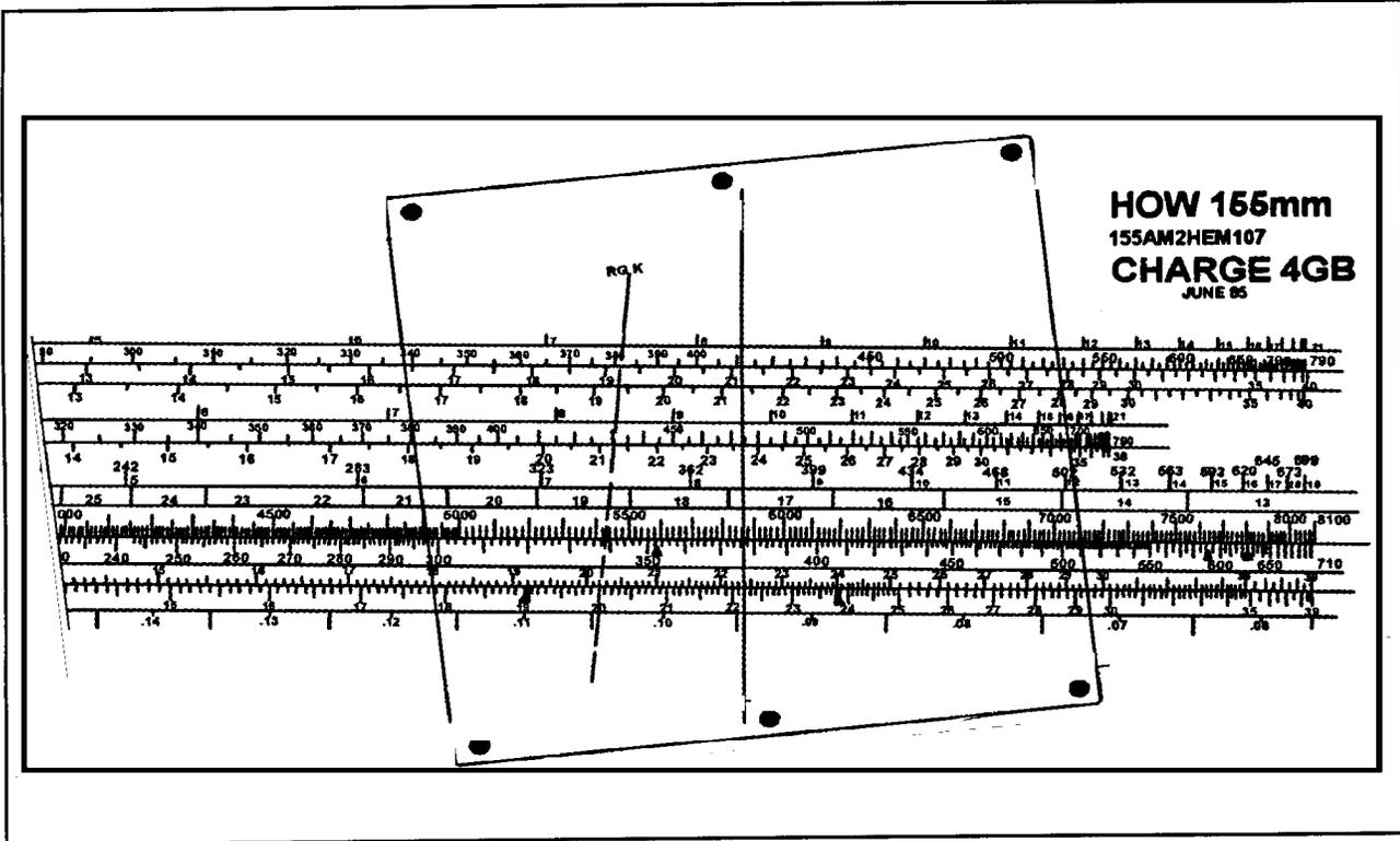
Figure 7-21. Graphical Firing Table.
