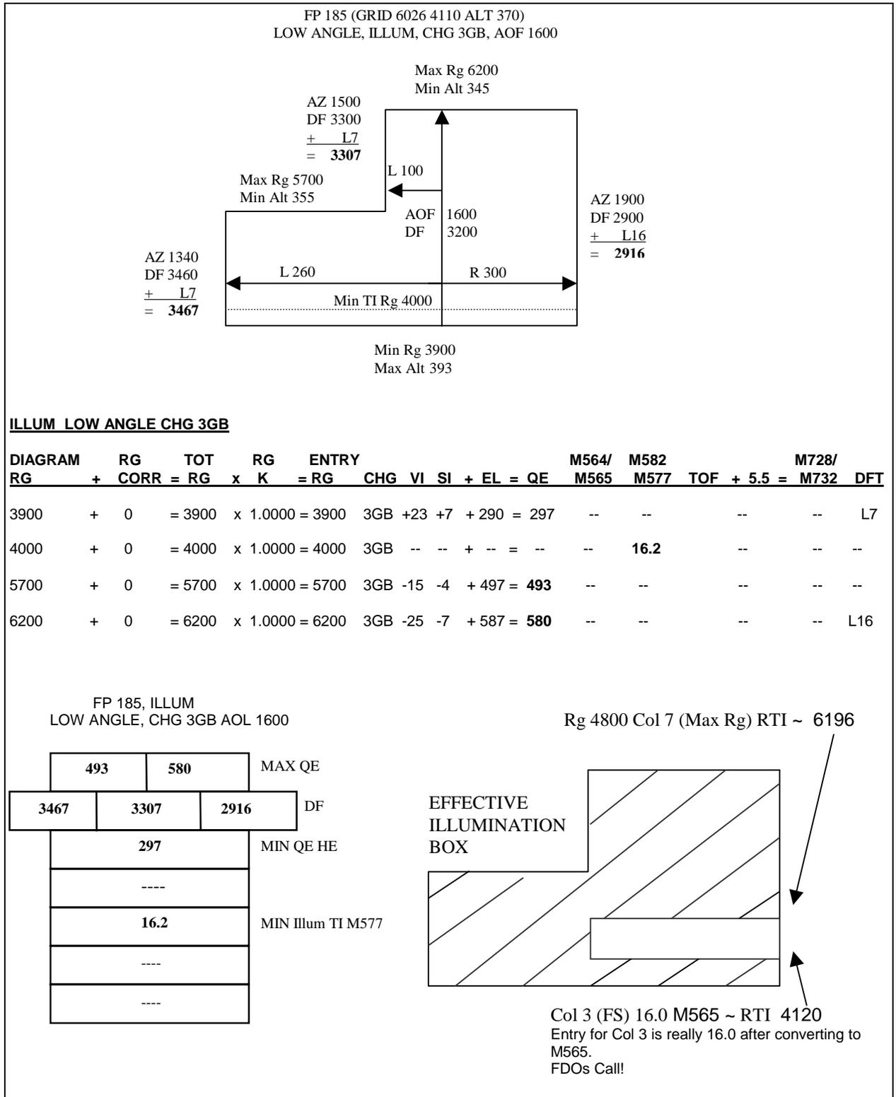
Figure 15-10. Example of Low Angle Safety, Shell Illum
