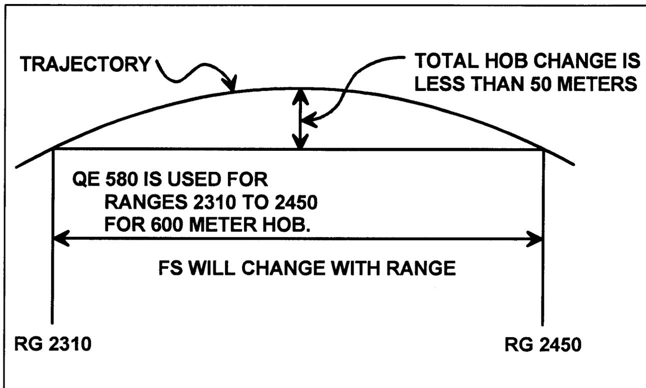
**Figure 7-24. Trajectory of an Illuminating Projectile, Charge 2GB.**
