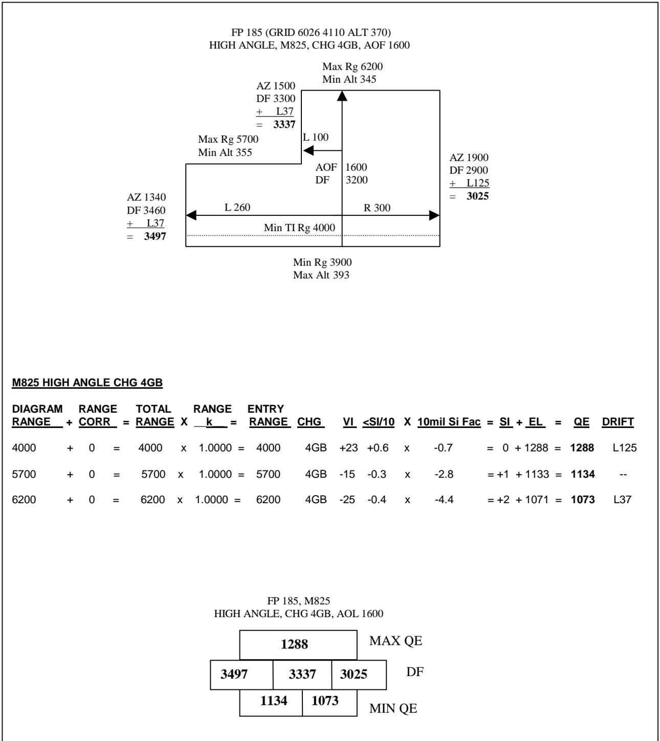
Figure 15-14. Example of High Angle Safety, Shell M825
