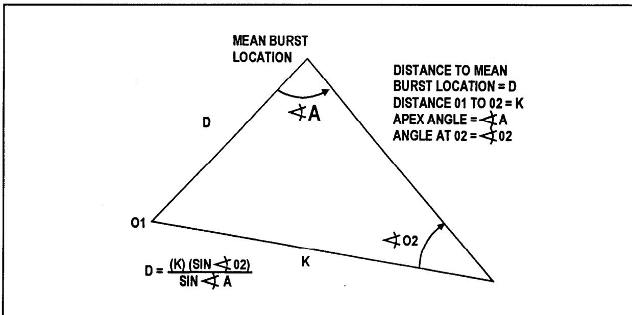
**Figure 10-13. Formula for Computing Distance to the MBL.**
