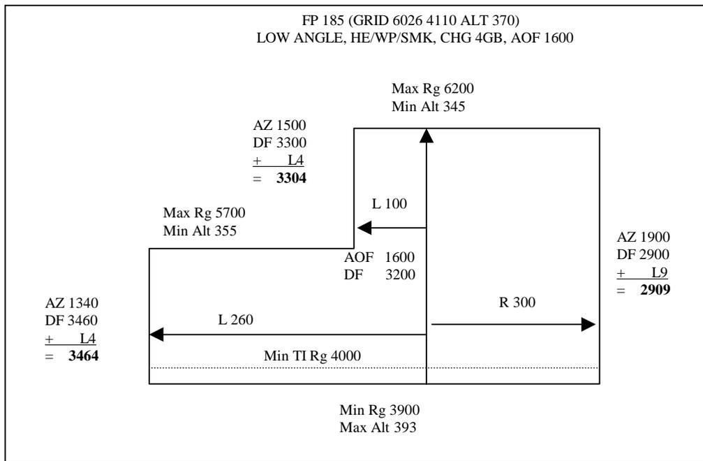
Figure 15-2. Example of a Completed Safety Diagram, HE/WP/SMK
