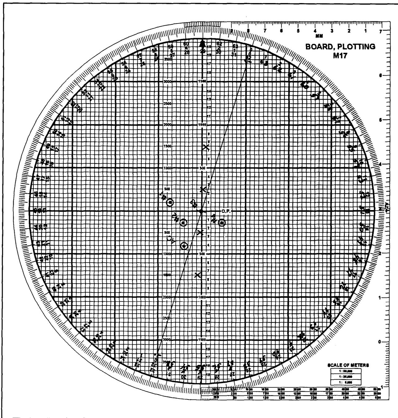
Figure 12-17. M17 Plotting Board Oriented on Altitude 1300, With Target and Burst Points Plotted.
