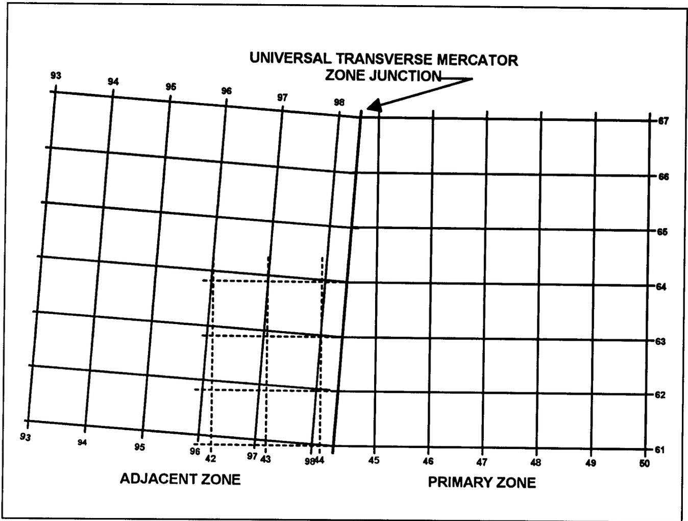
**Figure H-9. Joining Two Grid Sheets for Zone-To-Zone Transformation.**
