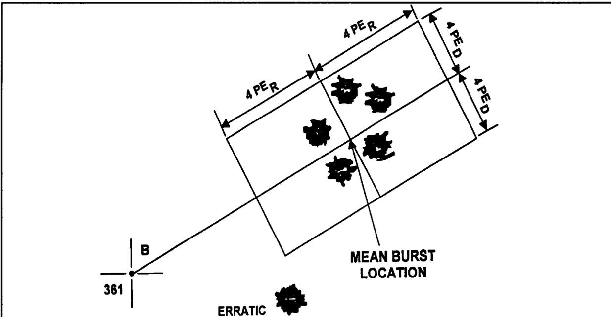
Figure 10-7. 8 PER x 8 PED Rectangle for HB Registration.
