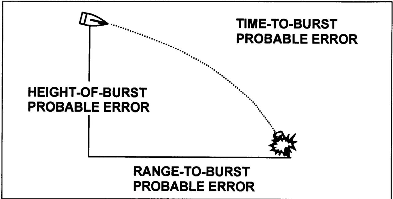
Figure 3-13. Comparison of PE<sub>HB</sub>, PE<sub>RB</sub>, and PE<sub>TB</sub>.
