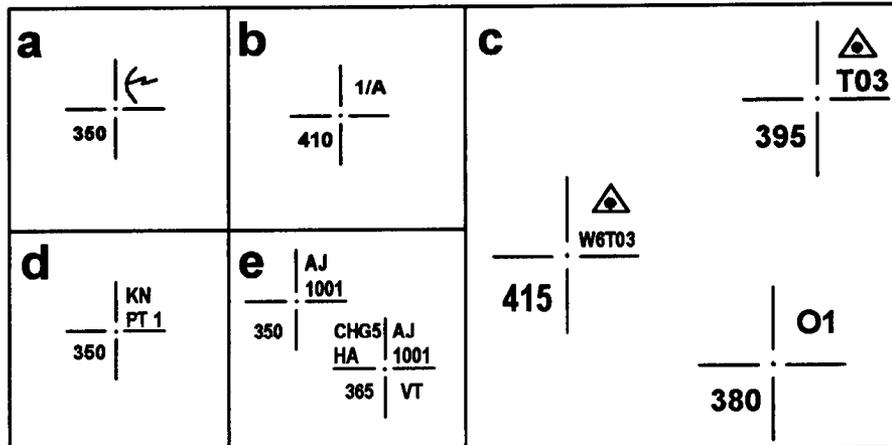
**Figure 6-12. Example of Different Tick Marks.**
