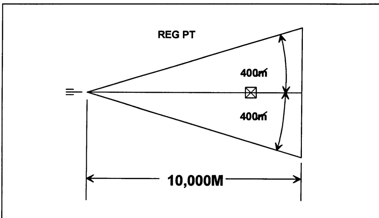
Figure 10-24. Deflection Transfer Limits--10,000 Meters or Less.
