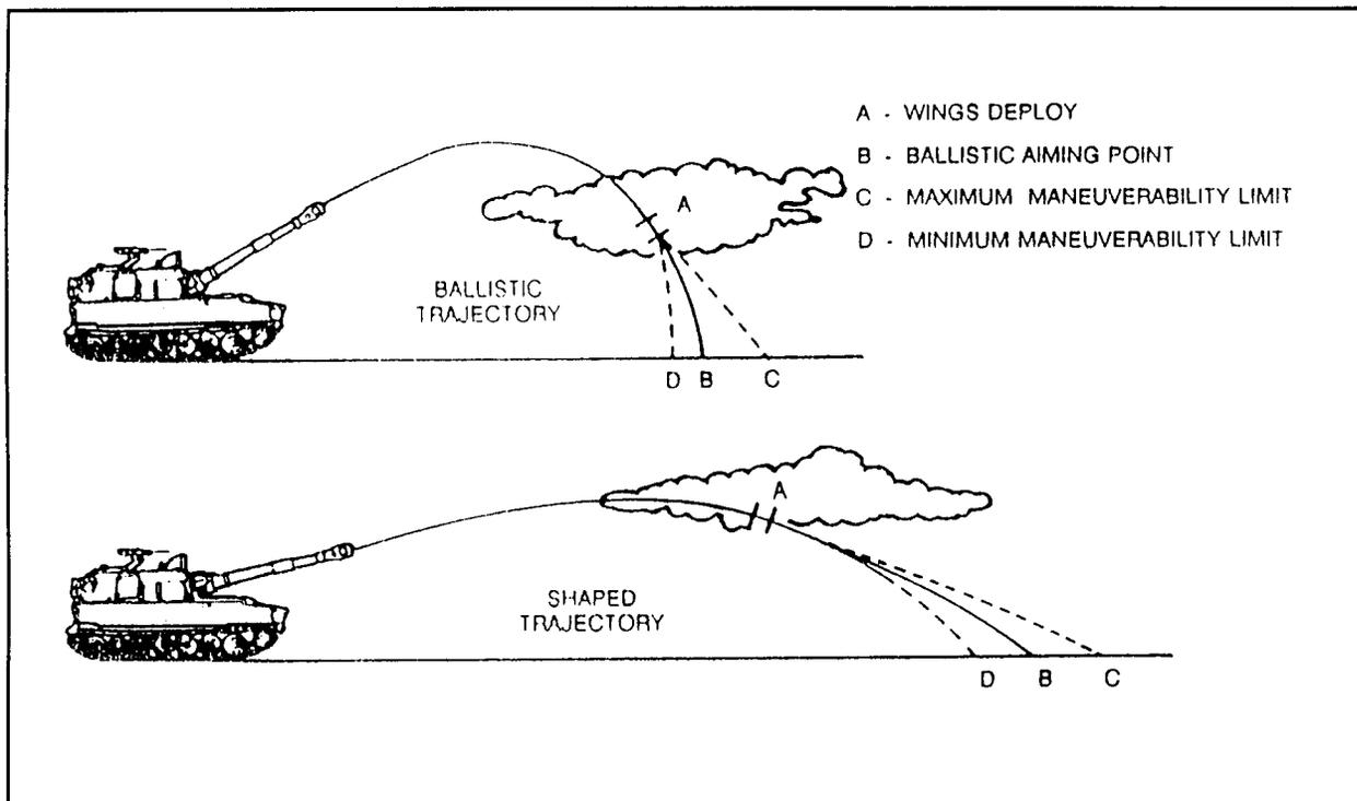
**Figure 13-3. Comparison of Low-Angle Ballistic Trajectory and Shaped Trajectory.**
