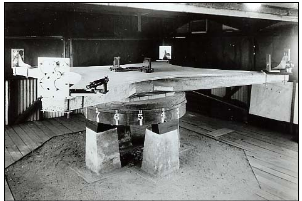
FIG. 7. Miller's Control Experiments. Top Photo: A wooden platform has been supplied for the mirrors and optics of the interferometer, inside a building at Case School. Bottom Photo: A concrete platform supports the mirrors and optics of the interferometer, inside a small shelter on the grounds at Case School.
