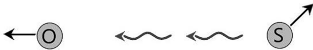
Fig. 1. Observer, Signal and Source: The velocity of a source does not influence the speed of a signal – but only the motion of the observer relative to the signal influences its time of flight.
