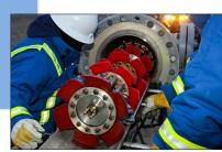
Pipelines deliver massive amounts of crude daily and ensuring safe operation is key. The EMCORE DSP-1760, coupled to additional sensors, provides these inspection robots with extremely accurate angular data.
