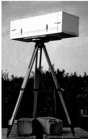
Figure 7. Interferometer at the measuring point
