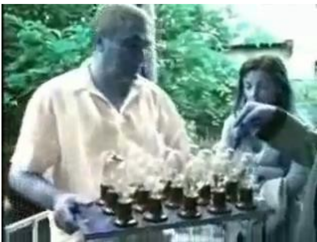
Figure 16. Load variant - incandescent lamps with total power of 3 kW.
