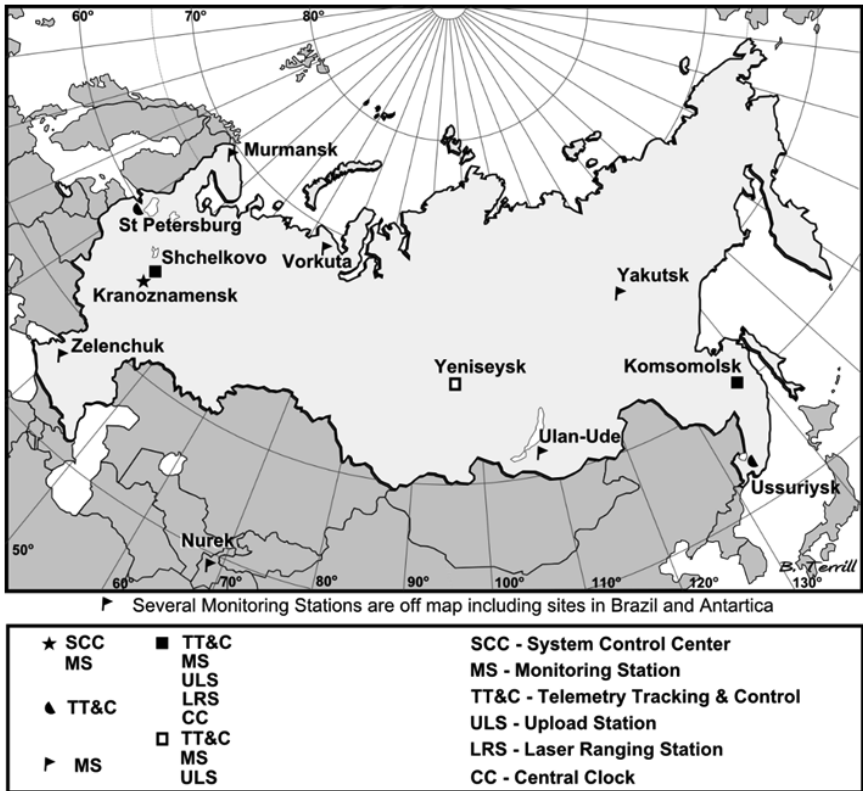
Figure 4.7 GLONASS ground segment.
