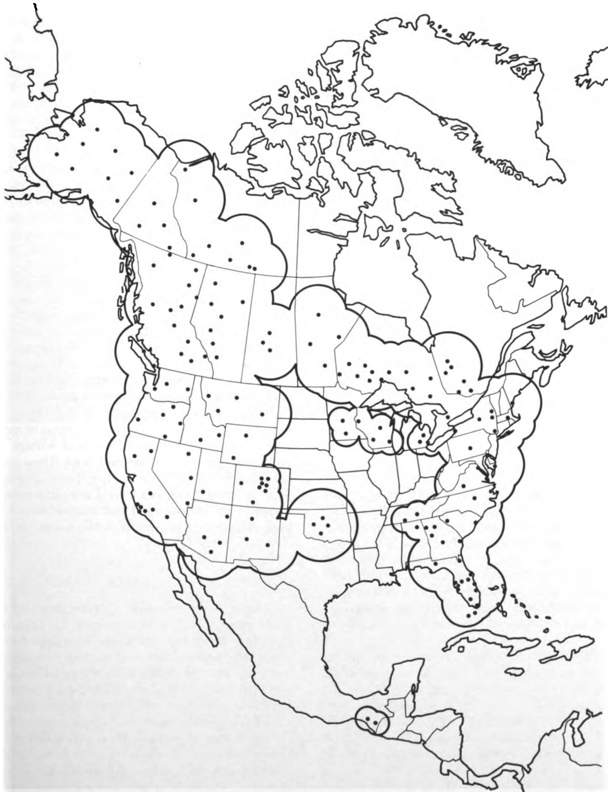
FIGURE 5.1 A map showing the location (dots) of lightning direction finding (DF) stations in place in summer 1984. Connected circles around each DF indicate area of lightning coverage. The area of coverage along the East Coast is the SUNYA East Coast Network.
