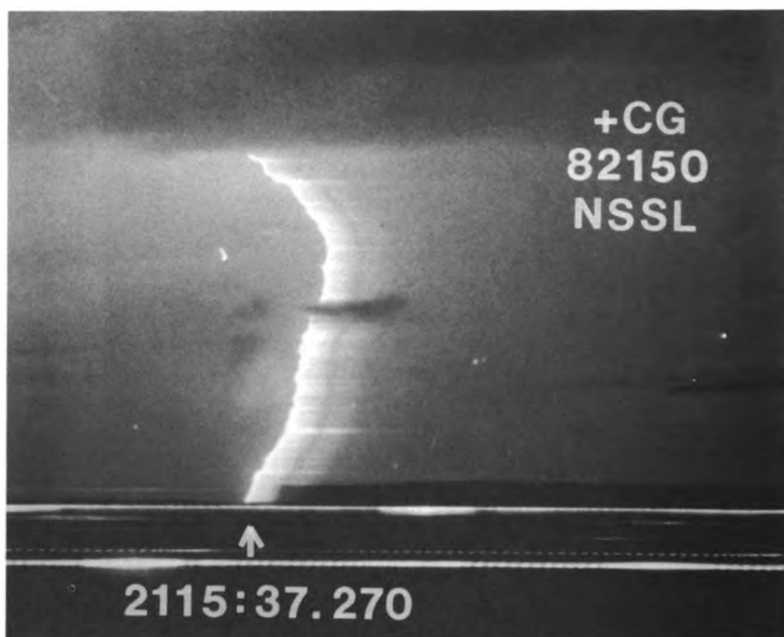
FIGURE 3.4 Streak-film photograph of +CG flash recorded on May 30, 1982 (see Figures 3.2 and 3.3). Continuing current is evident from the smearing of luminosity. It is visible in the photograph for about 60 msec and occurs during interval b in Figure 3.2.
