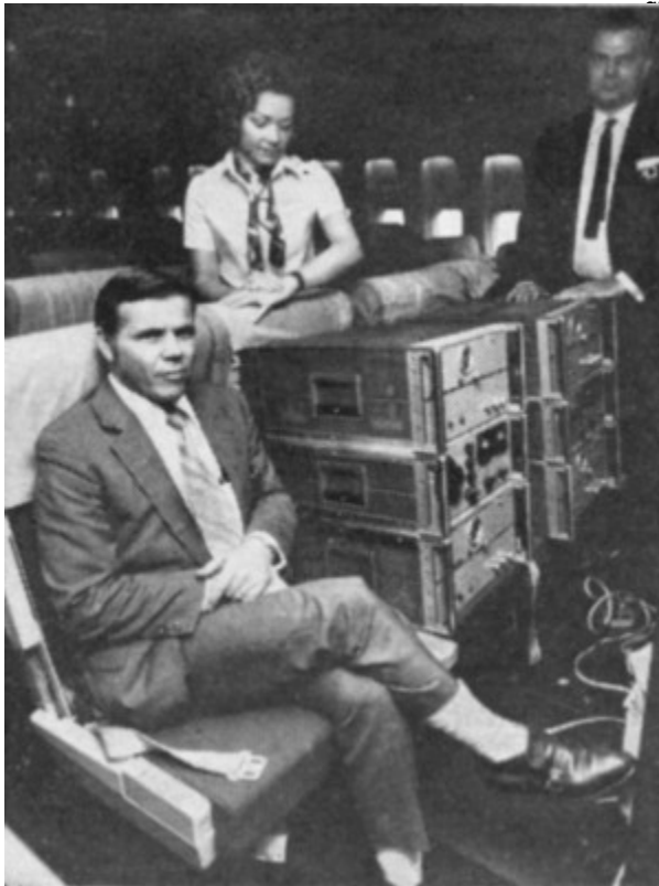
Physicists Joseph Hafele (b. 1933) and Richard Keating on board an airliner, with their cesium atomic clocks.
