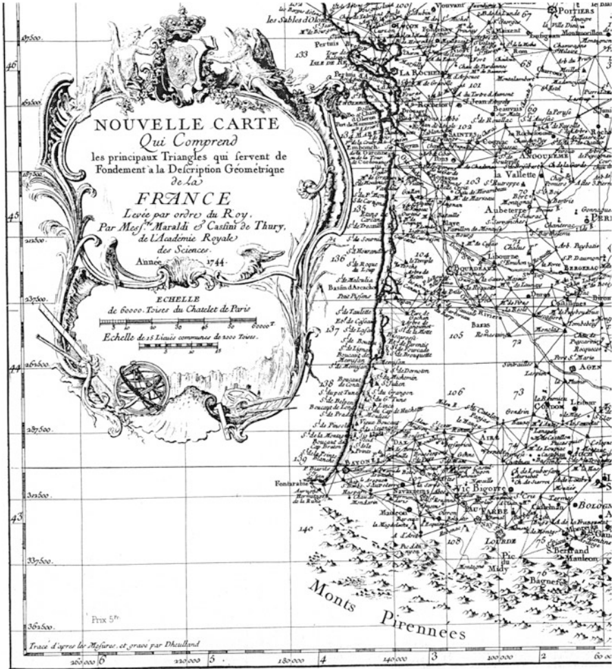
FIG. 2.8 : Map of France (by Maraldi and Cassini de Thury) 1744. Detail of frontispiece. This map shows the rays observed in building up the primary triangulation network. Cartographic projection: Cassini projection.
