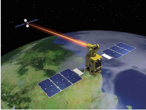
FIG. 9.36 : Artist's view of the laser link between the Japanese satellite OICETS and the European satellite Artemis. Credit: JAXA.
