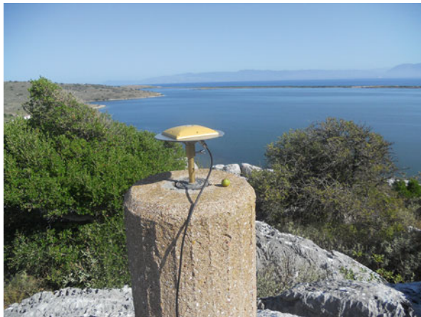
FIG. 14.25 : GPS beacon belonging to the network of the Corinth Rift Laboratory, near Galaxidi, Fokida, Greece, September 2012. Studying the region of high seismic activity in the Gulf of Corinth. Photo M.C.
