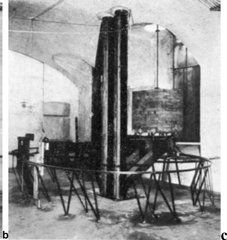
Fig. 8 – Majorana's second experimental setup (a) made use of a large lead cube PP as a gravitational shield. The test body M in the basement was attached to a balance H kept at the ground floor of the building. The two halves of the lead cube were supported by wood structures that could rotate around the pillar AB and be brought to the position P'P' . Measurements were made both with the test body surrounded by the lead cube and without it. The photographs show the actual arrangement, with the lead cube away from the test body (b) and enclosing it (c).
