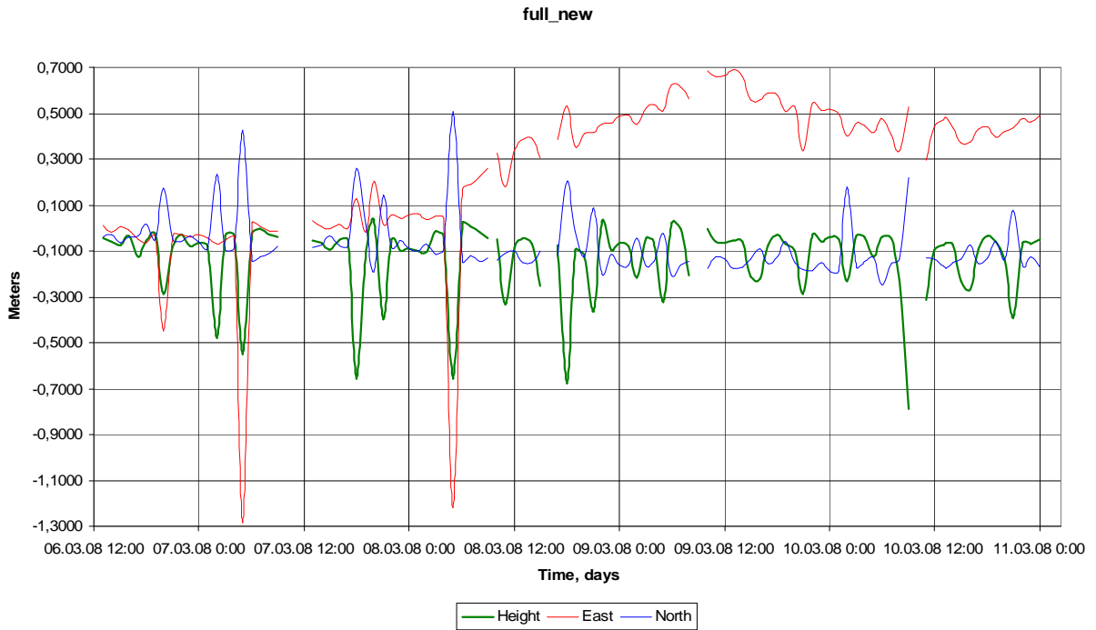
Figure 11. GPS measurement. Ice point “Balok” motion relative to coast point “Baza”, 12 h 06.03.2008 – 00h 08.03.2008. Seiche have 4÷5 h period.
