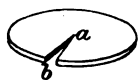
FIG. 6.— a represents a lead plate, of which the sector b is cut out.
