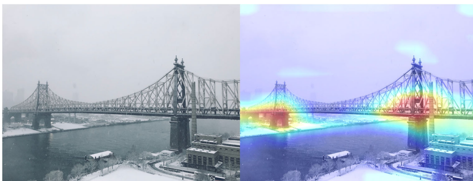
Fig. 14 An example of a class activation map (CAM) [58]. A CNN network trained on ImageNet classified the left image as a “bridge pier”. A heatmap for the category of “bridge pier”, generated by a method called Grad-CAM [59], is superimposed (right image), which indicates the discriminative image regions used by the CNN for the classification
