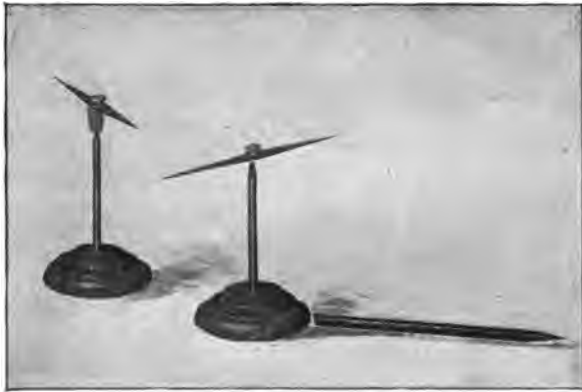
FIG. 2.—REPULSION BETWEEN LIKE POLES OF MAGNETIC NEEDLE.
