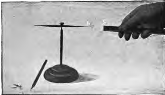
FIG. 3.—ATTRACTION BETWEEN ONE POLE OF A PIVOTED NEEDLE, AND THE POLE OF THE APPROACHED BAR MAGNET.
