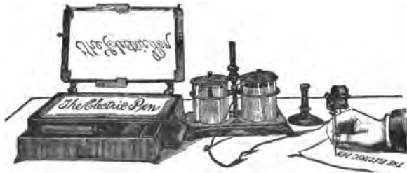
FIG. 59.—EDISON'S ELECTRIC PEN AND DUPLICATING PRESS.
