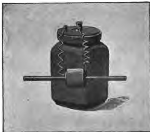
FIG. 40.—ELECTROMAGNETIC EFFECT OF AN ELECTRIC CURRENT PASSING THROUGH A COIL OF WIRE.
