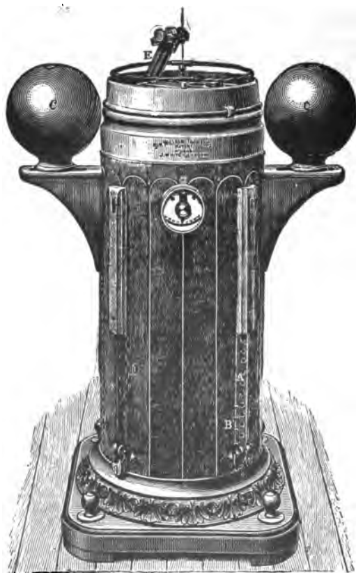
FIG. 98.—THOMPSON'S COMPENSATING BINNACLE.
