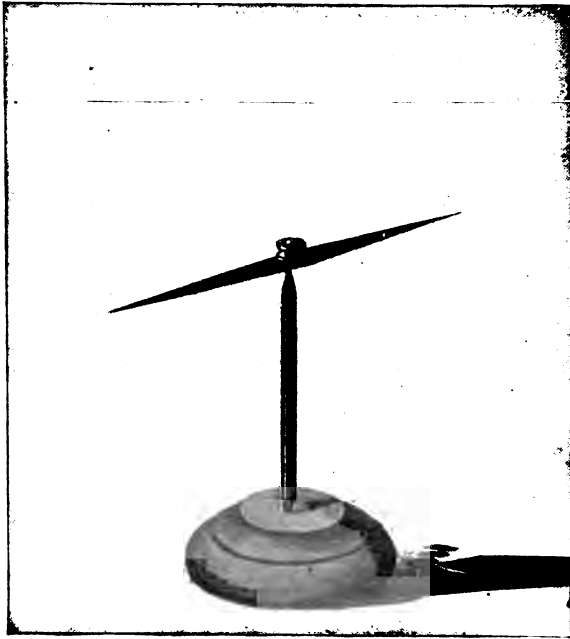
FIG. 29.—DEFLECTION OF MAGNETIC NEEDLE WHEN SUPPORTED BENEATH A WIRE CONVEYING AN ELECTRIC CURRENT.
