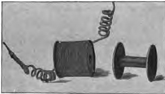
FIG. 39.—COIL OF WIRE WOUND ON INSULATING SPOOL.
