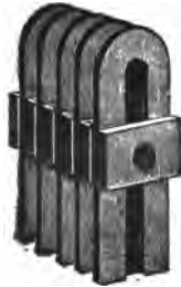
FIG. 53.—COMPOUND PERMANENT MAGNET EMPLOYED FOR THE REMOVAL OF IRON PARTICLES FROM WHEAT.
