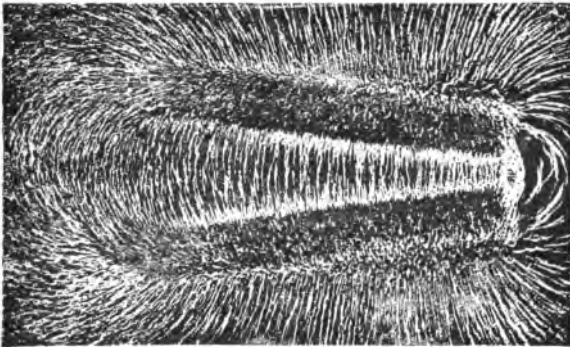
FIG. 19.—MAGNETIC FLUX OF HORSESHOE MAGNET.
