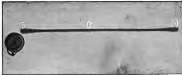
FIG. 7.—MAGNETIZED BAR WITH IRON FILINGS SHOWING POLAR CONDITION.
