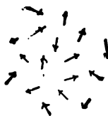
FIG. 10.—HETEROGENEOUS ASSOCIATION, CORRESPONDING TO ABSENCE OF MAGNETIZATION.
