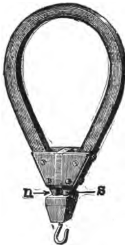
FIG. 49.—COMPOUND PERMANENT MAGNET WITH CONSTANT POLE SURFACES.
