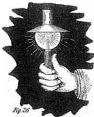
FIG. 26.—INCANDESCENCE OF A SOLID.—ILLUSTRATING FOUR KINDS OF LIGHT EFFECTS PRODUCED BY HIGH FREQUENCY CURRENTS OF HIGH POTENTIAL.
