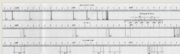
Fig. 8.7 Homologies in the spectra of magnesium, zinc, and cadmium: a refers to singlets, c to doublets, b to triplets, d to quartets, and e to quintets. From Hartley [1883 b ] pl. 1. Note that the scale refers to “oscillation frequencies” in units of 10 oscillations per mm.
