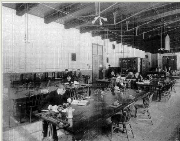
Fig. 9.1 General physics laboratory, MIT Boston campus, in the 1890s. Students performing exercises, one with a microscope and one with a prism spectroscope and a small heliostat mirror. Reproduced by permission of the MIT Museum, Department Photo Albums, vol. 24, no. 10.
