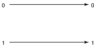
FIGURE 1.3. Noiseless binary channel. C = 1 bit.
