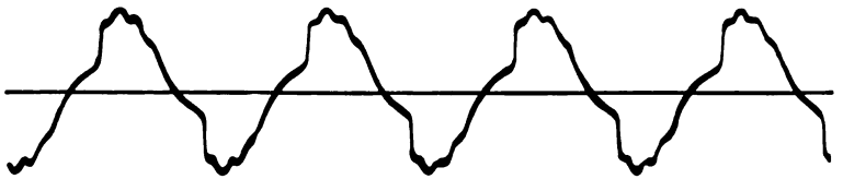
Fig. 68. Secondary terminal e.m.f. of transformer.
