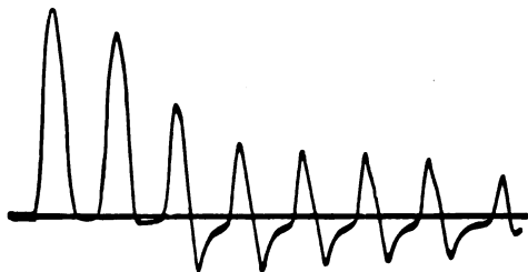
Fig. 47. Starting current of a 25-cycle transformer.
