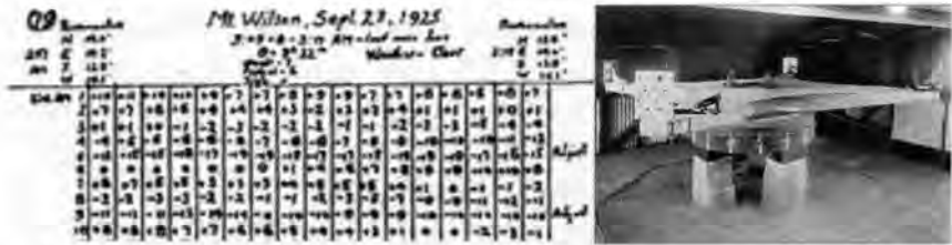
Figure 3. Left: upper part of Miller's data sheet for run No. 79. Temperature readings of four thermometers located at N, E, S, W in the room were read at the beginning of the run at 03:09 (left upper corner), and at 03:17 (right upper corner). Right: Miller's Control Experiments. A concrete platform supports the mirrors and optics of the interferometer, inside a small shelter on the grounds at Case School.
