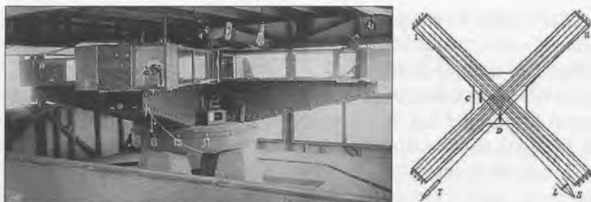
Figure 1. Miller's interferometer (left). Light paths of the Michelson-Morley and Miller Interferometers, as seen from above (right).
