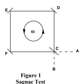
Figure 1 shows a schematic representation of the test. A source at 'A' sends light to a half-silvered mirror at C. Some of the light goes from C to D, E, F and C and is reflected to an observer at B. Some of the light goes around the other way. The whole apparatus (including A and B), turns with an angular speed of  $\omega$ . The difference in time (dt) for the light to traverse the path, in opposite directions, was derived by Sagnac as:
