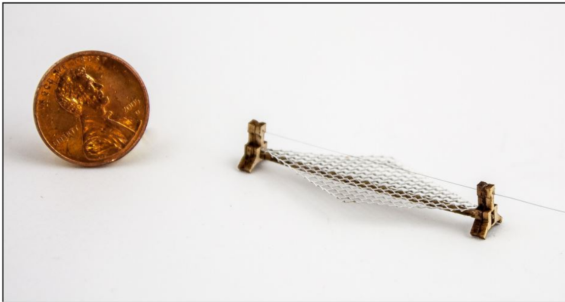
Figure 3.2: Fabricated meso-scale ionocraft. Components: Tungsten wire ( 50\mu\text{m} diameter), aluminum mesh, balsa wood frame.
