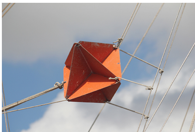
Figure 1.11 A radar reflector hoisted on a sailboat is a type of corner reflector. (credit: Tim Sheerman-Chase)
