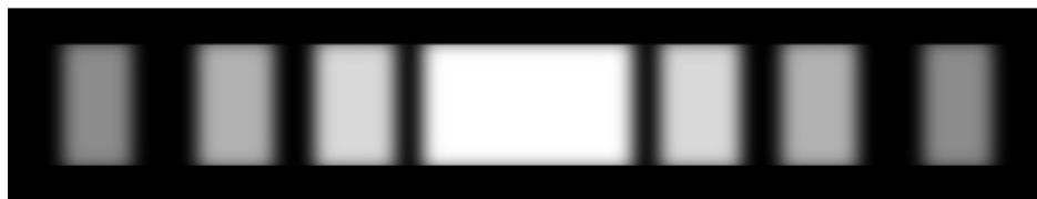
Figure 4.9 (a) The calculated intensity distribution of a single-slit diffraction pattern. (b) The actual diffraction pattern.
