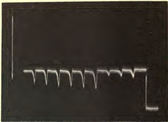
FIG. 7.—RECORD OF RESPONSES IN PLANT (LEAF-STALK OF CAULIFLOWER) BY METHOD OF NEGATIVE VARIATION
