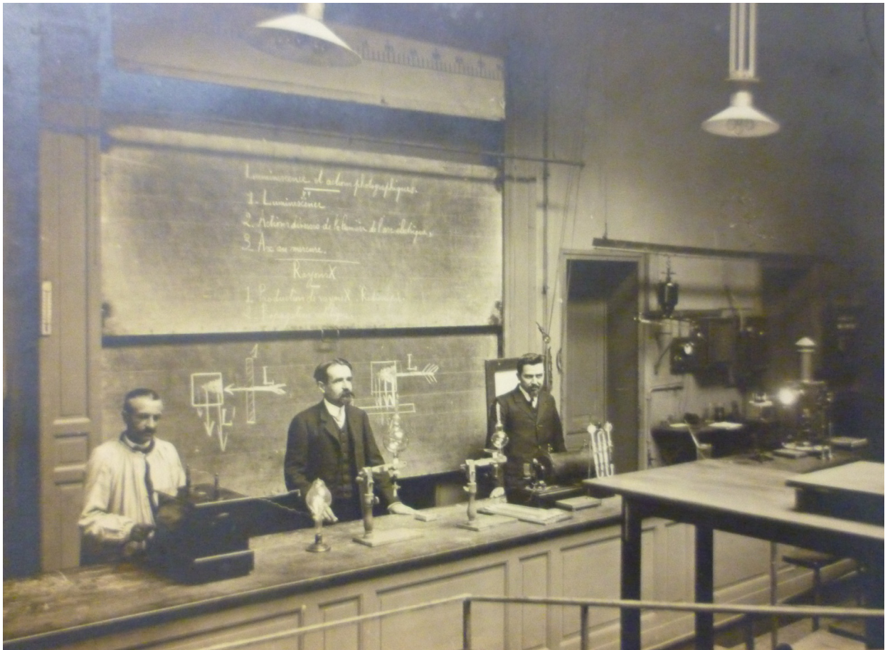
Fig. 6. Sagnac teaching (with two assistants on his sides). From the inscription on the blackboard, it appears that Sagnac was teaching luminescence, photographic action, X-rays, and transformed rays in the same lesson. The two drawings illustrate the permutation of scatterer and absorber as a proof of transformation (probably for light, as the letters L and L' suggest). X-ray tubes and Ruhmkorff coils can be seen on the desk. The lamp on the right corner may be part of setup for showing the transformation of light by a solution of fluorescein. From Archives nationales.
